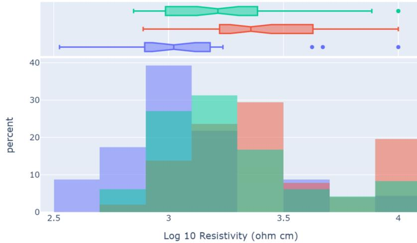
**Figure 5:** The Variation of Soil Resistivity Among Different Pipelines
