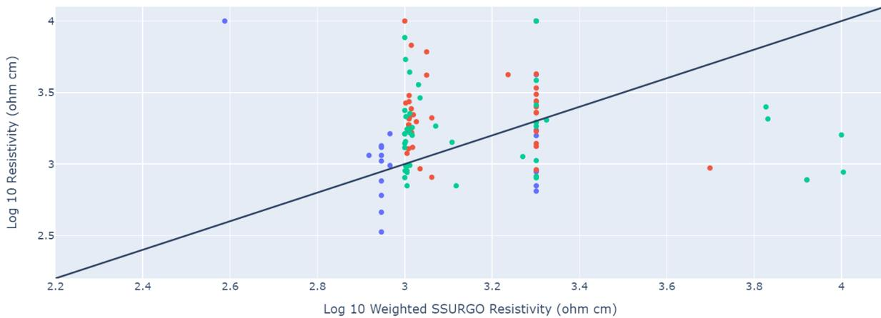
**Figure 6:** Field Validation of SSURGO Electrical Conductivity (green: Line 1, red: Line 2, and green: Line 3)
