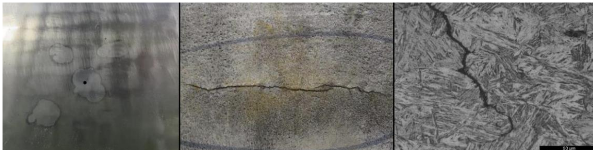
Figure 31 Hard spot containing martensite exhibiting cracking
