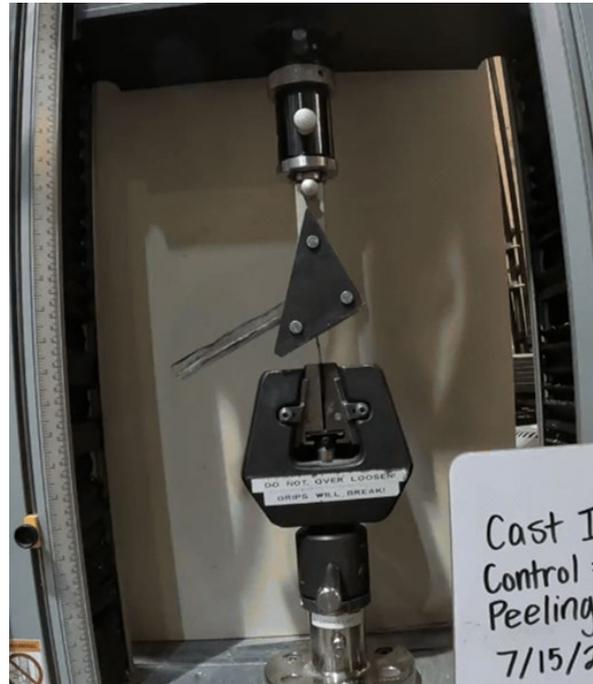
Figure 7.18: Peel Test Setup
