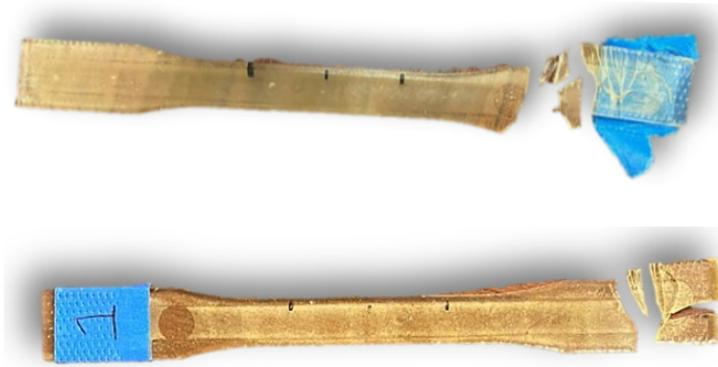
**Figure 4.10: Specimens after tensile test**
