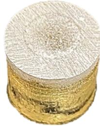
**Figure 5.14: Compressive test specimen after sanding**
