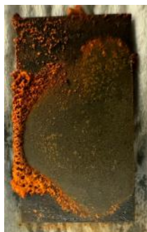
Figure 1.20. Corroded samples with a pectin film by dip-coating after 6 weeks
