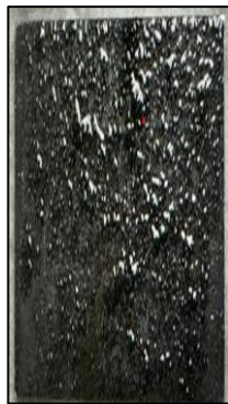
Figure 1.22. Corroded samples with a NMDEA film by dip-coating after 6 weeks
