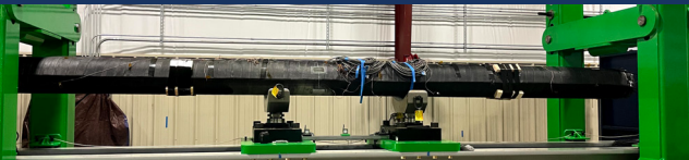
DFOS instrumented gas pipeline testing
