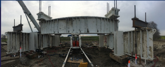
Testing of DFOS system for performance monitoring of bridge foundation piles (with Caltrans)
