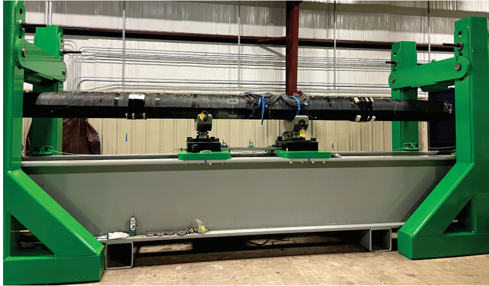
Figure 10: Instrumented pipe in four-point bending apparatus
