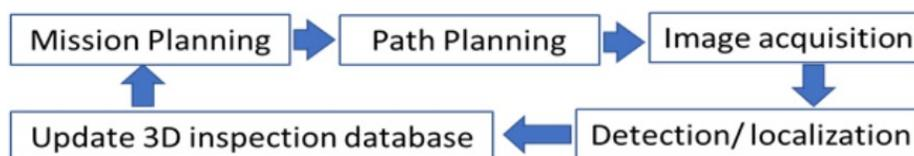
**Figure 1 Iterative UAS pipeline facility inspection procedures**
