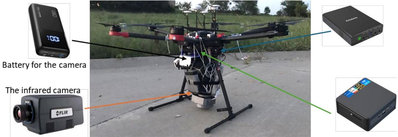
**Figure 43. Basketball net mounted UAS data acquisition system**
