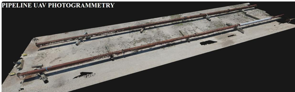
Figure 24. The point cloud model interface of PRCI field pipelines using UAS based photogrammetry.
