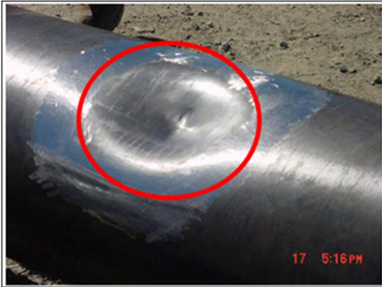
Figure 1 Picture of pipeline dent (Source: <https://www.google.com/imghp?hl=en>)
