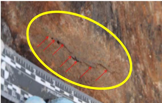
(c) In-service failure, dent @1.6% deep, **very rough, corroded profile**, restrained/unrestrained, (365psi max), failed at [12k cycle](#).
