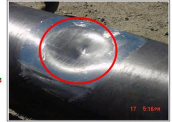
Figure 1 Picture of pipeline dent (Source: <https://www.google.com/imghp/3b/en>)
