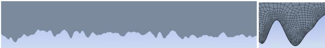
Figure 17: Random roughness shape (left) and its meshing detail (right).
