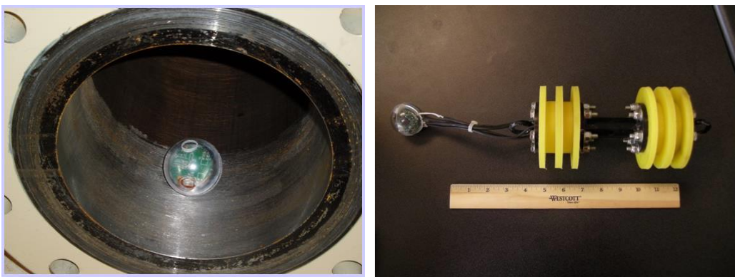
Figure 1.1. Examples of ball sensors that can move along the gas stream
