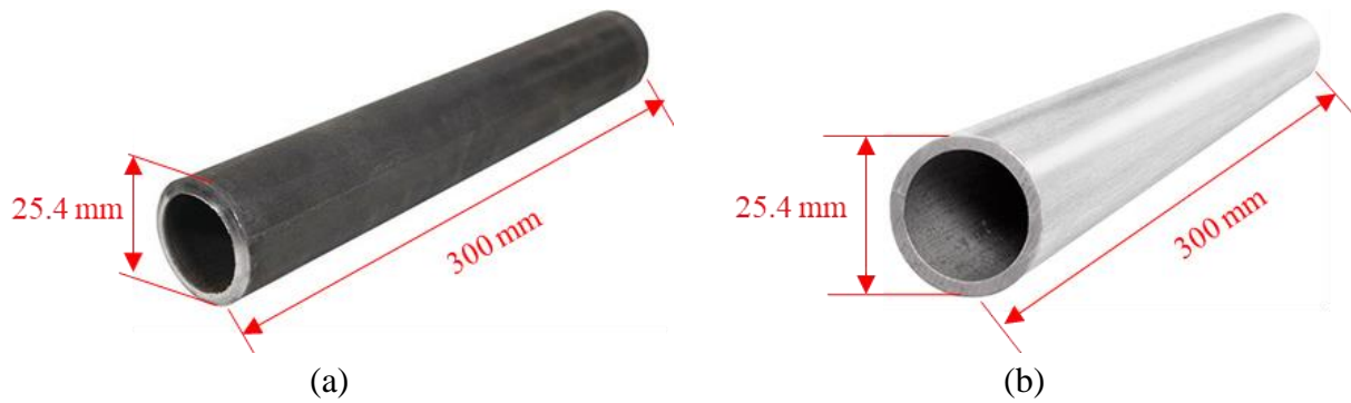
Figure 2.6.1. Pipe specimens: (a) a low-carbon steel pipe; and (b) a stainless steel pipe.
