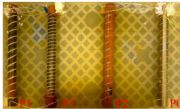
Figure 2.6.4. Four pipes immersed in a sodium chloride solution for corrosion experiments.
