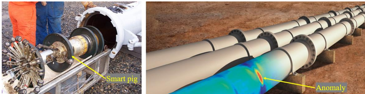
Figure 1.1.2. A smart pig travels along a pipeline and detects anomalies in the pipeline with use of the NDE tools incorporated in the smart pig.
