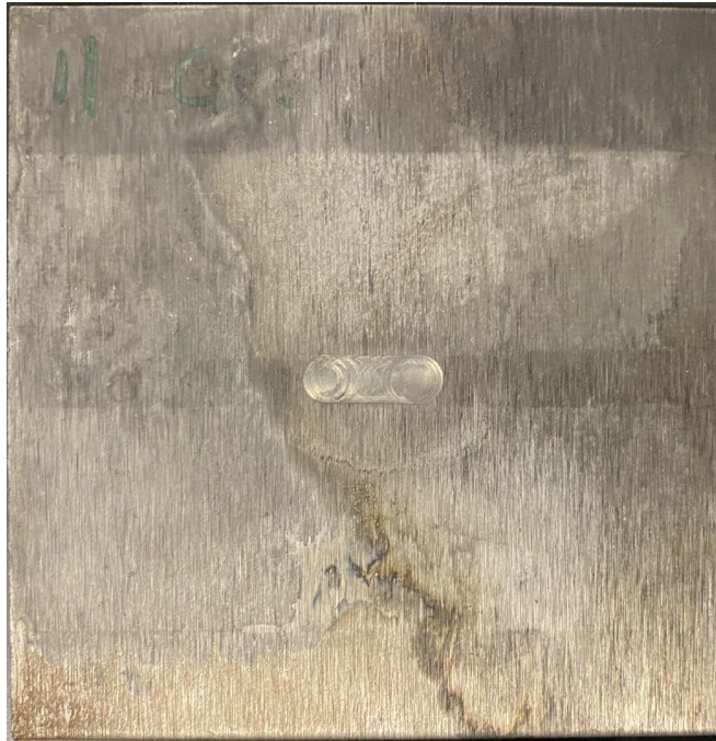
Figure A6. The pre-damaged steel sample before the exposure testing.
