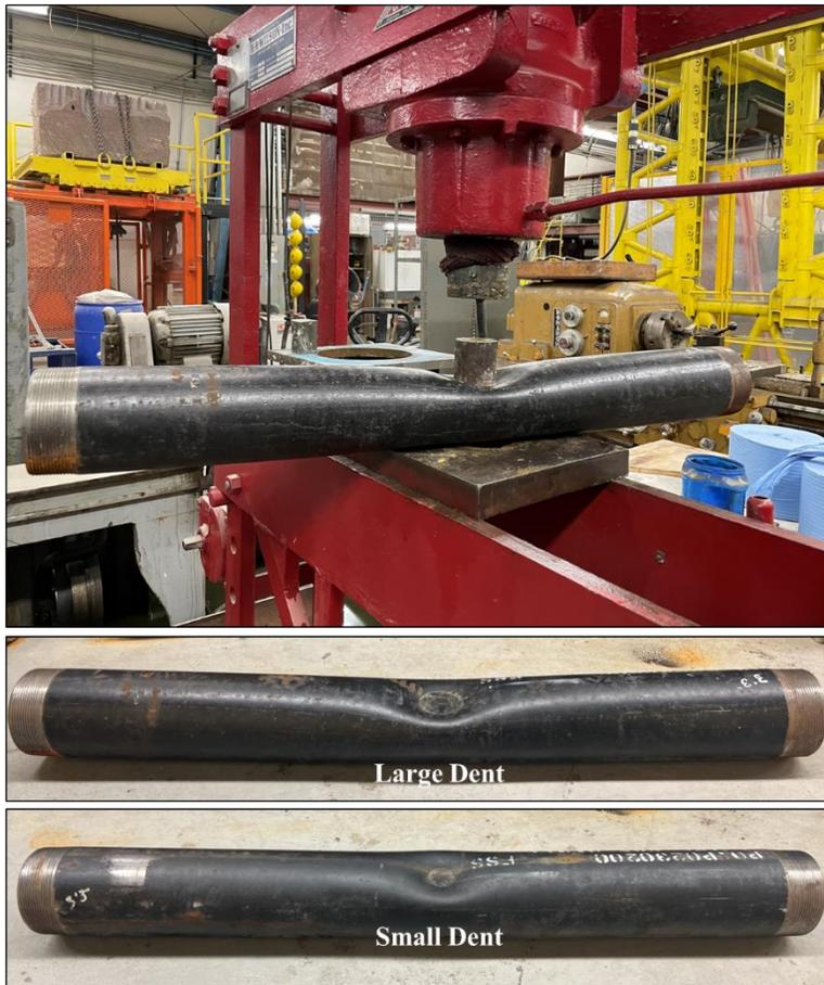
Figure 7. Photograph of the facility that created the dents and the 1-m test sections with two dent sizes.
