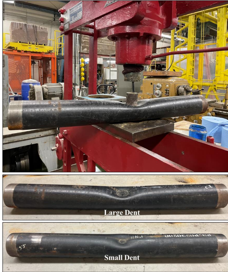
Figure 18. Photograph of the facility that created the dents and the 1-m test sections with two dent sizes.
