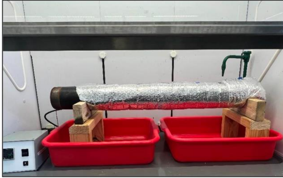
Figure 7. Photograph of the 1-m steel pipe during an ongoing lab corrosion preparation
