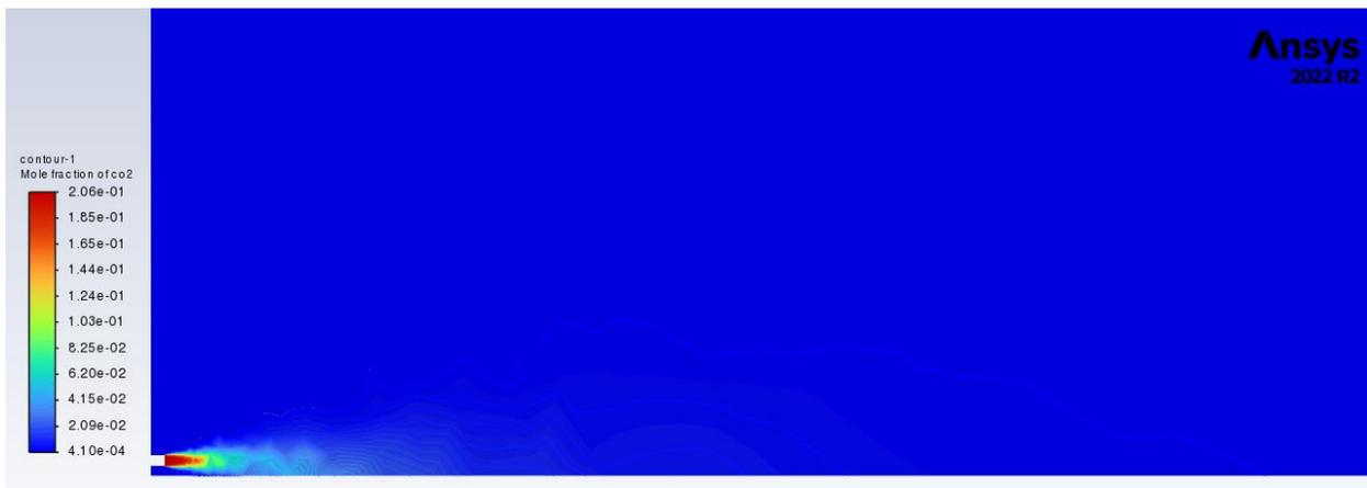
Figure 9. CO<sub>2</sub> concentration contours.
