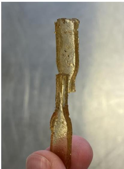
Figure 23. Weldability of the partially UV curable formulation.
