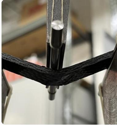
Figure 9. Three-point bending flexural property tests
