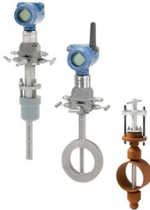
Figure 10 – Emerson Rosemount Annubar averaging pitot tube in single mount insertion, wafer, and opposite side support in severe service design. The single mount and wafer designs include an integral valve manifold and the differential pressure transmitter (courtesy of Emerson)
