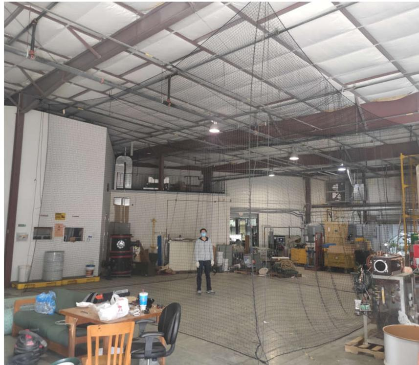
10 m × 8 m × 6 m drone net for control testing,
