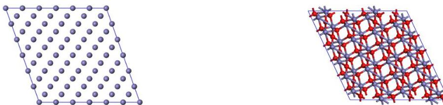
Figure 8. Atomistic surface models for Fe (110) (left) and Fe<sub>2</sub>O<sub>3</sub> (right). Both literature and our preliminary MD simulation results suggest that epoxy resin has a stronger interaction with the Fe<sub>2</sub>O<sub>3</sub> surface.
