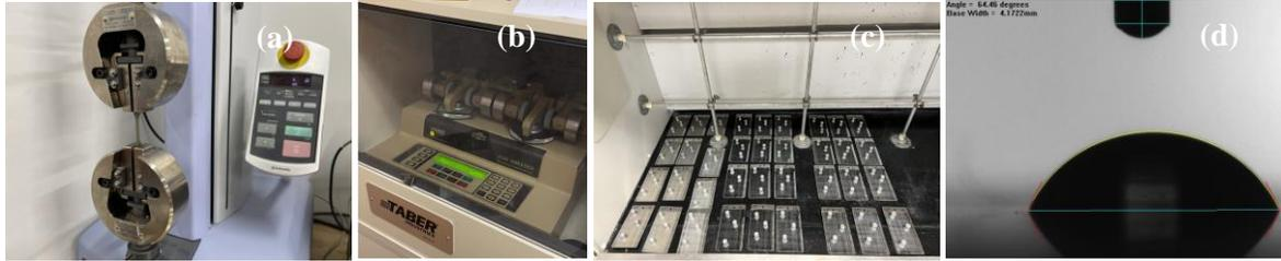
Figure 4. Testing setup for (a) coupon tensile test, (b) abrasion resistance test, (c) adhesion test, and (d) water contact angle test
