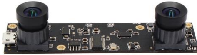
Figure 2.2: Dual Lens Aptina AR0330 USB Camera
