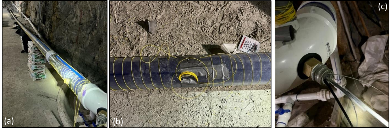
Fig. 1. (a) Photograph of the clear PVC section for Tasks#1 & 2 with helically wrapped cable (yellow) and straight cable covered by blue tape. Sand bags and moving blankets are used to prevent vibration and protect cable. (b) Photograph of a splice at a damaged point in the helically wrapped fiber. (c) Photograph of the sealing for internal cable deployment located at the entrance of the Orica drift in Edgar Mine. All cables are permanently deployed using epoxy compound. Flat and thin cables are damaged at this location.
