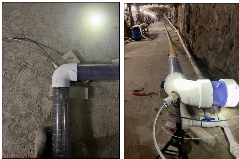
Figure 3. Photographs, left, Sealing using for internal cables at the end of the PVC section. Right, sealing for internal cable at the entrance of PVC test section.
