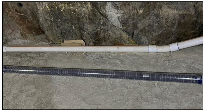
Figure 2. Photograph of section of clear PVC pipe with wrapped cable (yellow) and 3 cm of spacing in between.
