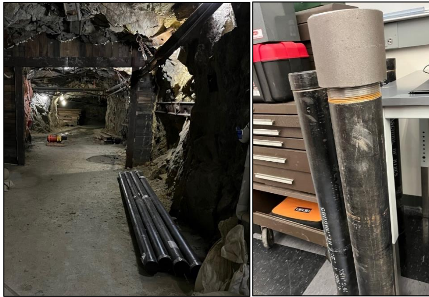
Figure 4. Left, Photograph of carbon steel pipes in Edgar Mine (API 5L X65 schedule 40 4-in, 5 m long each); Right, Photograph of 1-m section of steel pipe with a coupling at the top to connect in the middle of the pipeline
