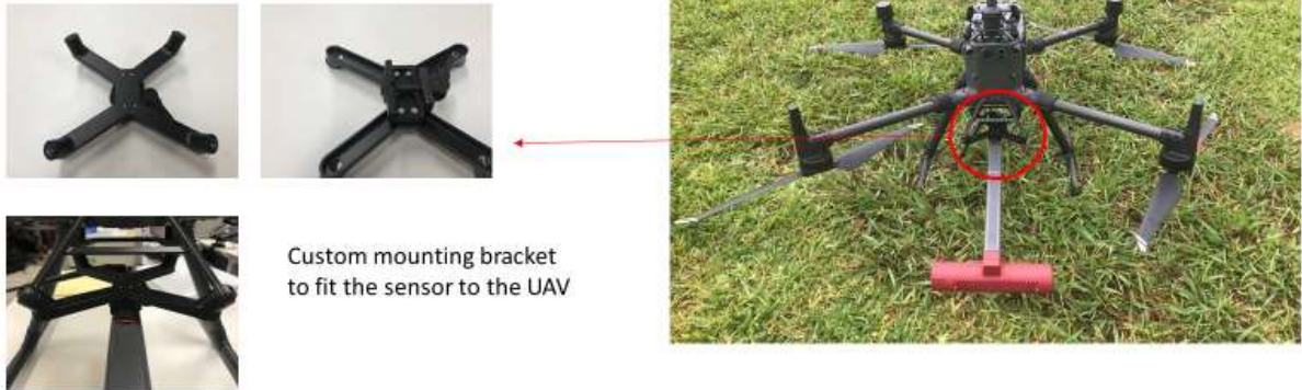
Figure 4. Camera and Methane Sensor Drone Mounting Configuration
