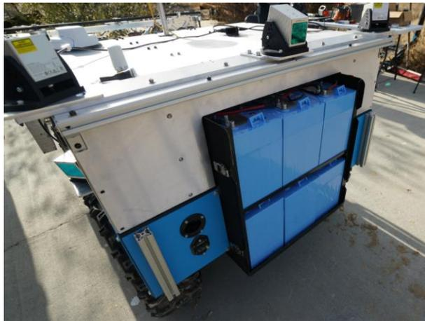
Figure 18: Back Side of Robot: Showing Batteries
