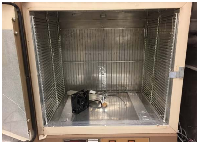
Figure 14. Test chamber used in evaluating the RMD devices
