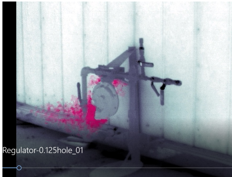
Figure 34. Gas Leak Image of the American Regulator, with hole and closed outlet
