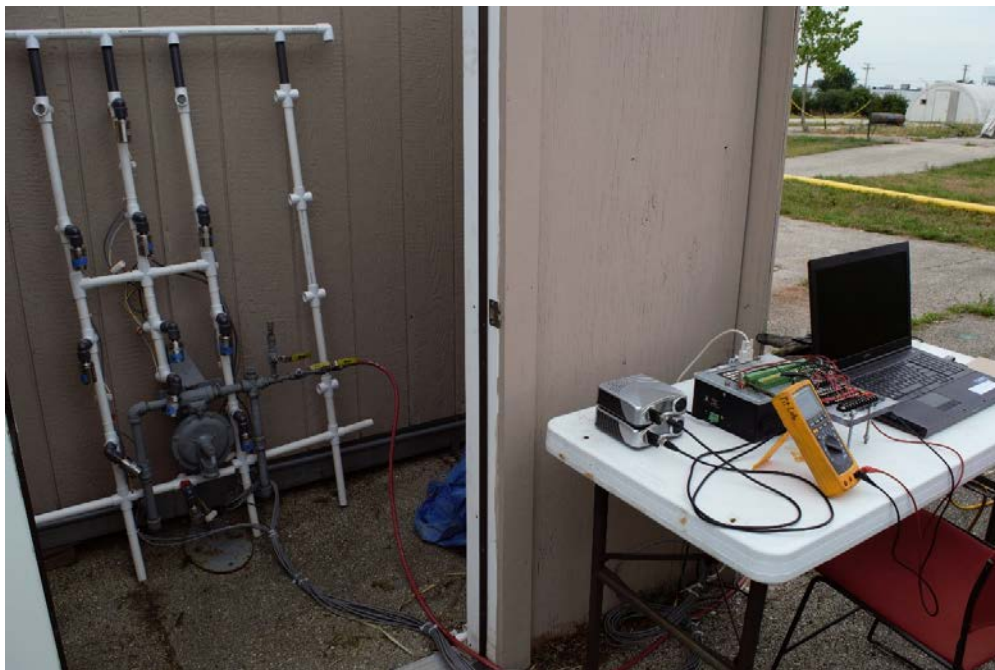
Figure 35. Sensors' setup and data collection system
