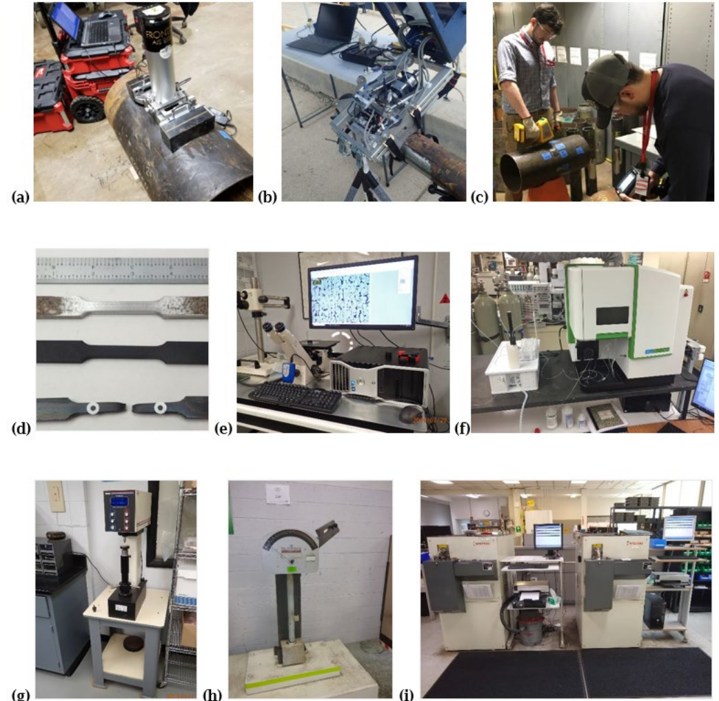
(a) Frontics AIS, (b) MMT HSD, (c) SciApps HH LIBS-OES, (d) Tensile Bars, (e) Grains Size Computer, (f) Lab ICP-OES Chemistry, (g) Hardness Tester, (h) Charpy Small Hammer, (i) OES Units.
