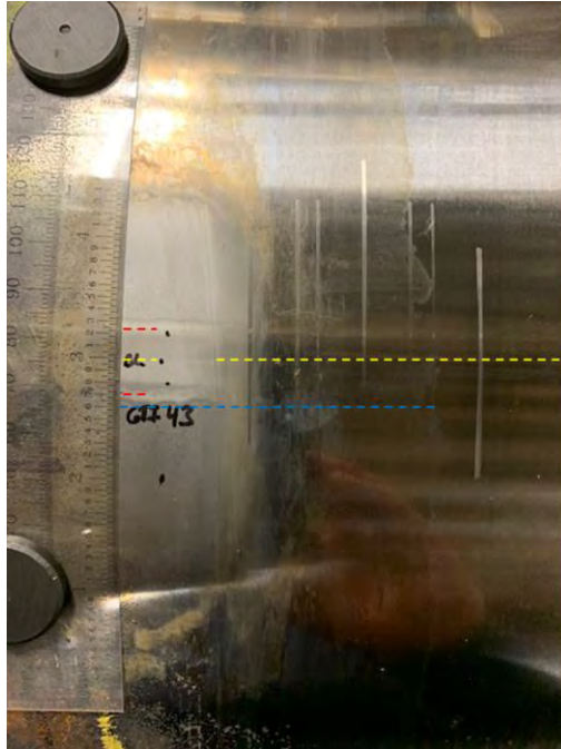
Figure 8: Examination of etched heat-affected-zone (HAZ) on the outer surface of the ERW seam for Sample 043. The bondline is located approximately 0.4 inches from the start of the HSD test.
