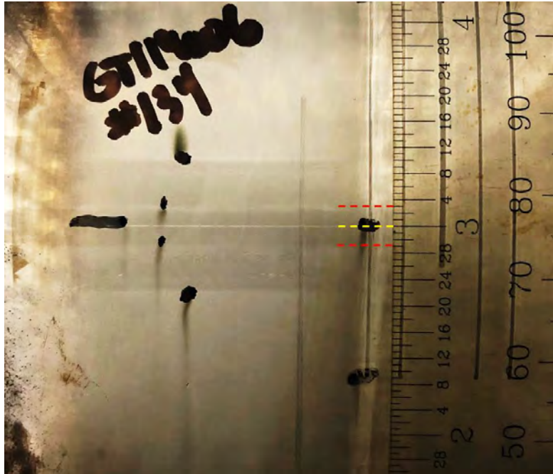
Figure 34: Examination of etched heat-affected-zone (HAZ) on the outer surface of the ERW seam for Sample 134. The boundaries of the etched HAZ are shown in dashed red lines and the bondline is shown by the dashed yellow line. The normalized HAZ width (measured width / wall thickness) is approximately 0.1875 \text{ in} / 0.26 \text{ in} = 72\% . The bondline is located approximately 0.6875 inches from the start of the HSD test.
