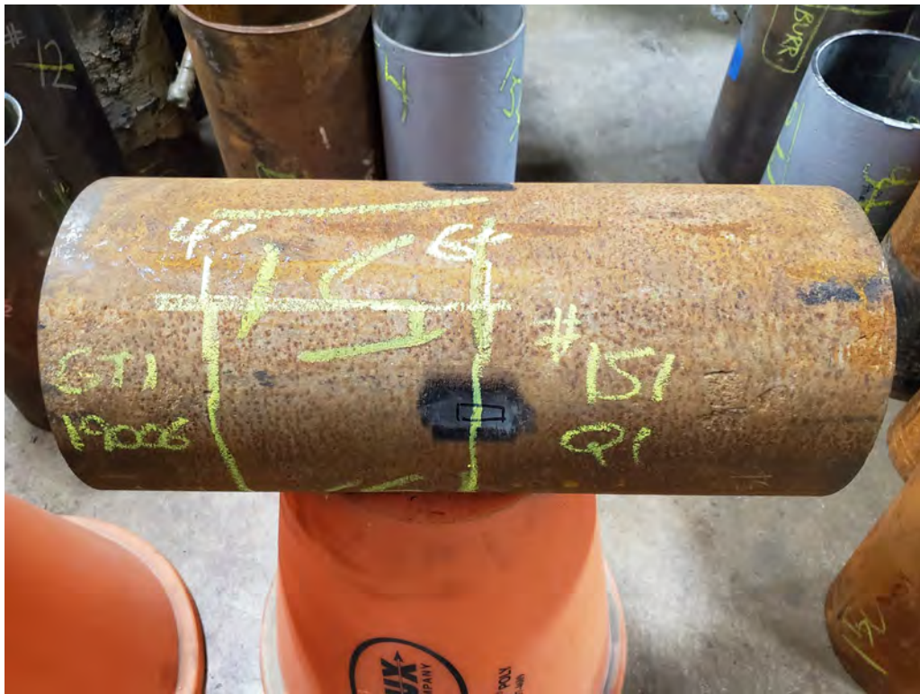
Figure 65: Test locations and overview of Sample 151.
