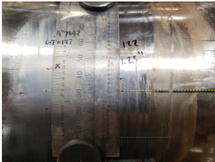
Figure 25: Examination of etched heat-affected-zone (HAZ) on the outer surface of the ERW seam for Sample 122. The bondline is located approximately 1.25 inches from the start of the HSD test.
