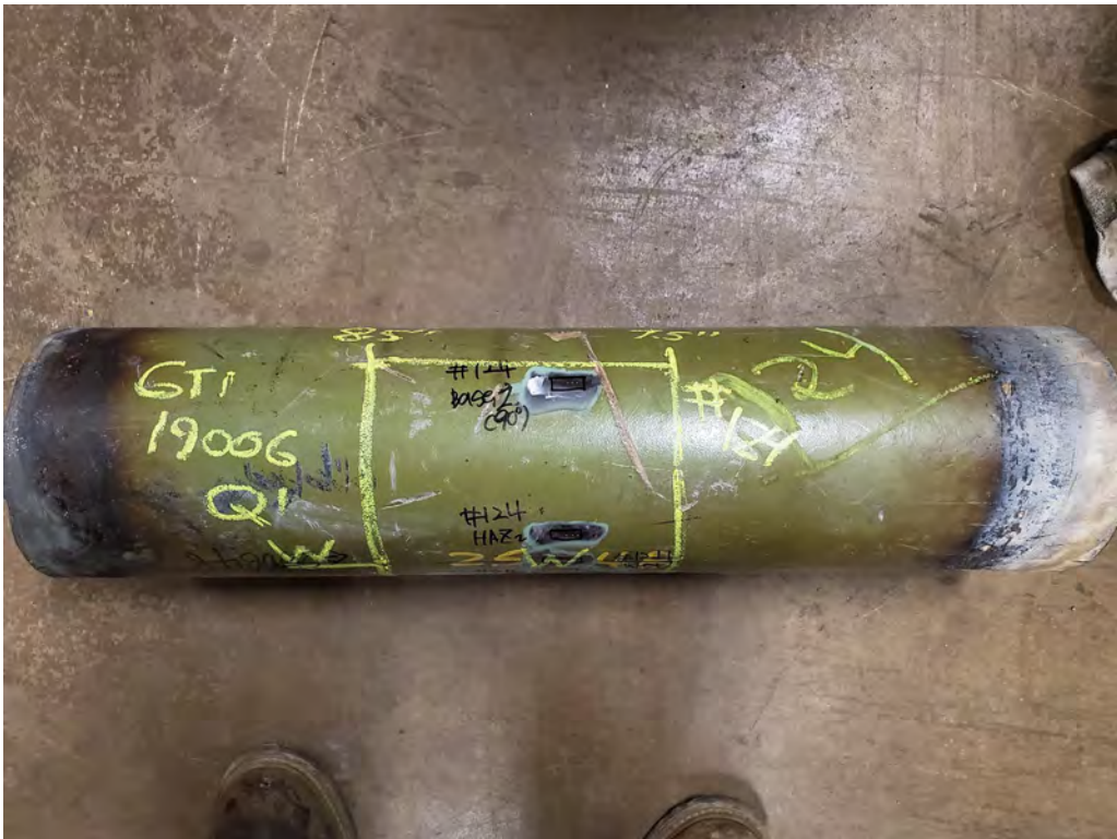
Figure 42: Test locations and overview of Sample 124.
