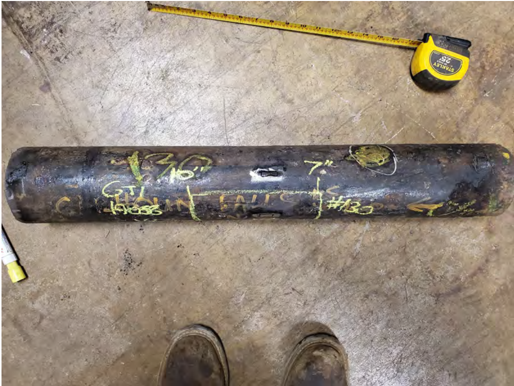
Figure 46: Test locations and overview of Sample 130.
