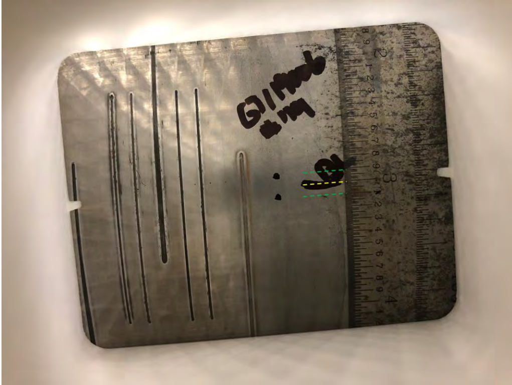
Figure 22: Examination of etched heat-affected-zone (HAZ) on the outer surface of the ERW seam for Sample 119. The edges of an inner hourglass HAZ surrounding the bondline are shown by the dashed green lines and the bondline is shown by the dashed yellow line. There is no presence of a larger, outer HAZ as a result of a normalization process indicative of HFN-ERW seams.
