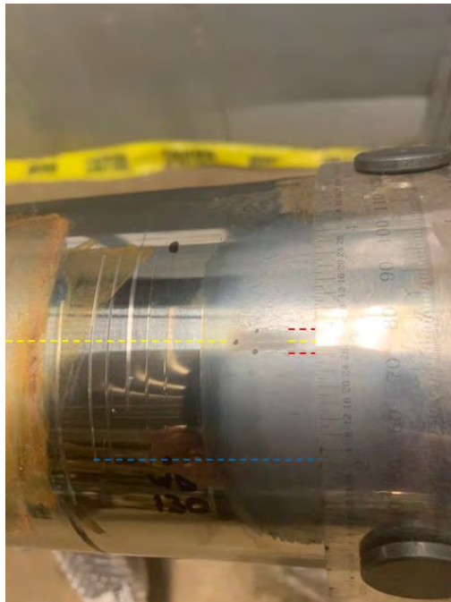
Figure 31: Examination of etched heat-affected-zone (HAZ) on the outer surface of the ERW seam for Sample 130. The bondline is located approximately 1.0 inch from the start of the HSD test.
