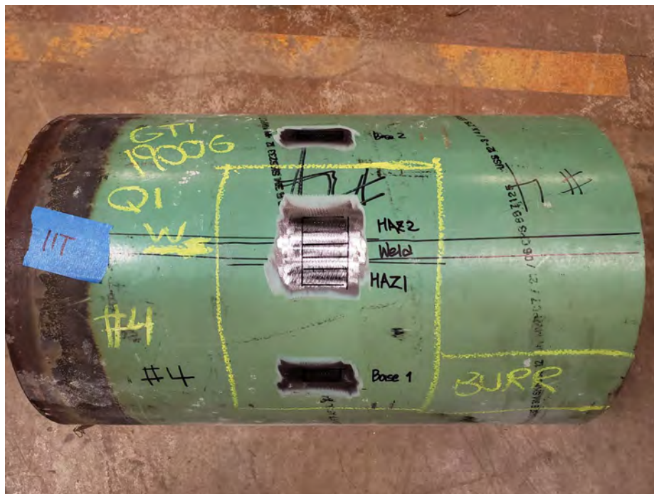
Figure 2: Test locations and overview of Sample 004.
