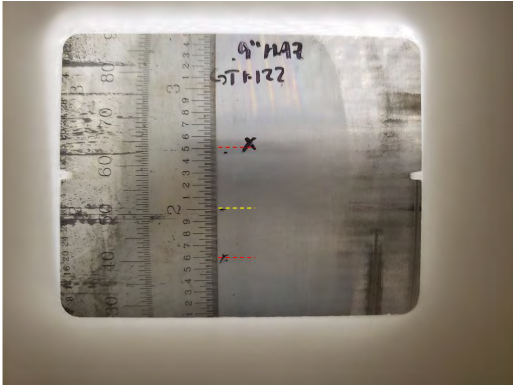
Figure 24: Examination of etched heat-affected-zone (HAZ) on the outer surface of the ERW seam for Sample 122. The boundaries of the etched HAZ are shown in dashed red lines and the bondline is shown by the dashed yellow line. The normalized HAZ width (measured width / wall thickness) is approximately 0.90 \text{ in} / 0.25 \text{ in} = 357\% .
