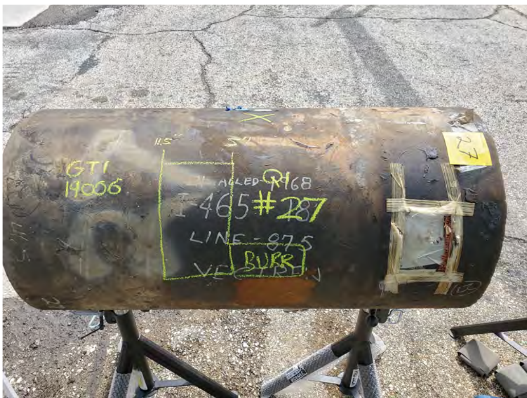
Figure 12: Test locations and overview of Sample 027.
