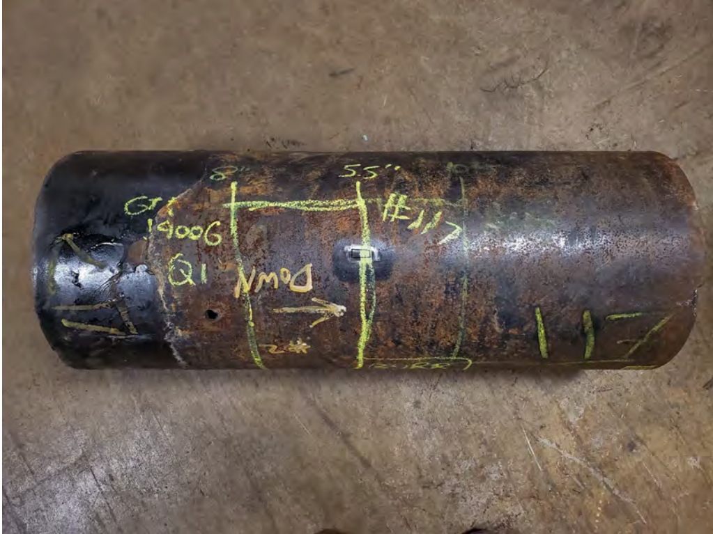
Figure 36: Test locations and overview of Sample 117.
