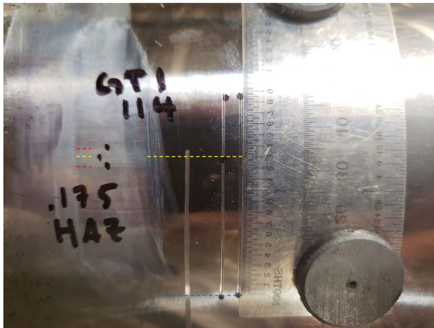
Figure 17: Examination of etched heat-affected-zone (HAZ) on the outer surface of the ERW seam for Sample 114. The bondline is located approximately 1.3 inches from the start of the HSD test.
