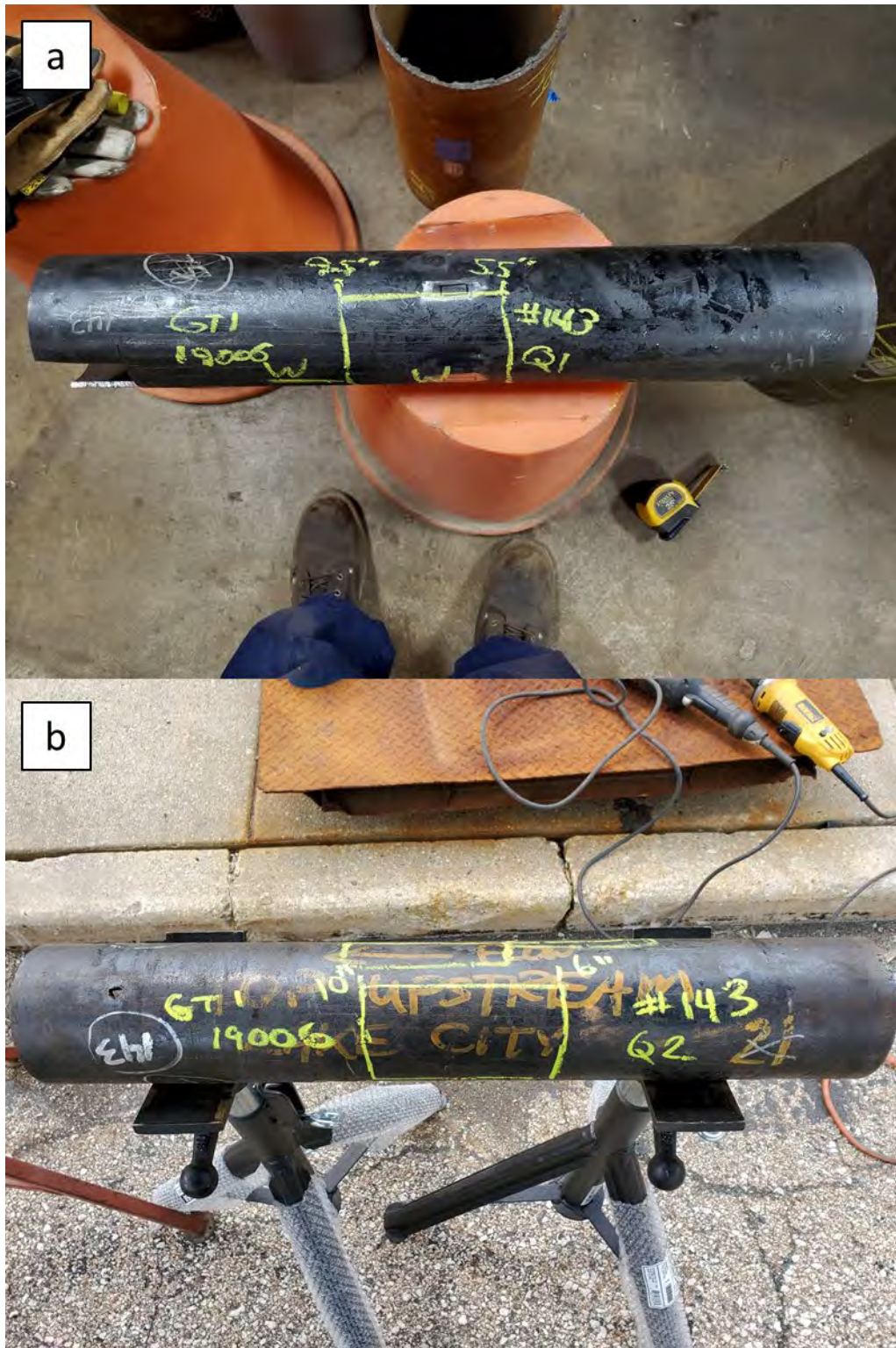
Figure 57: (a) Test location Q1 on ERW seam and overview of Sample 143; (b) Test location Q2 and overview of Sample 143.
