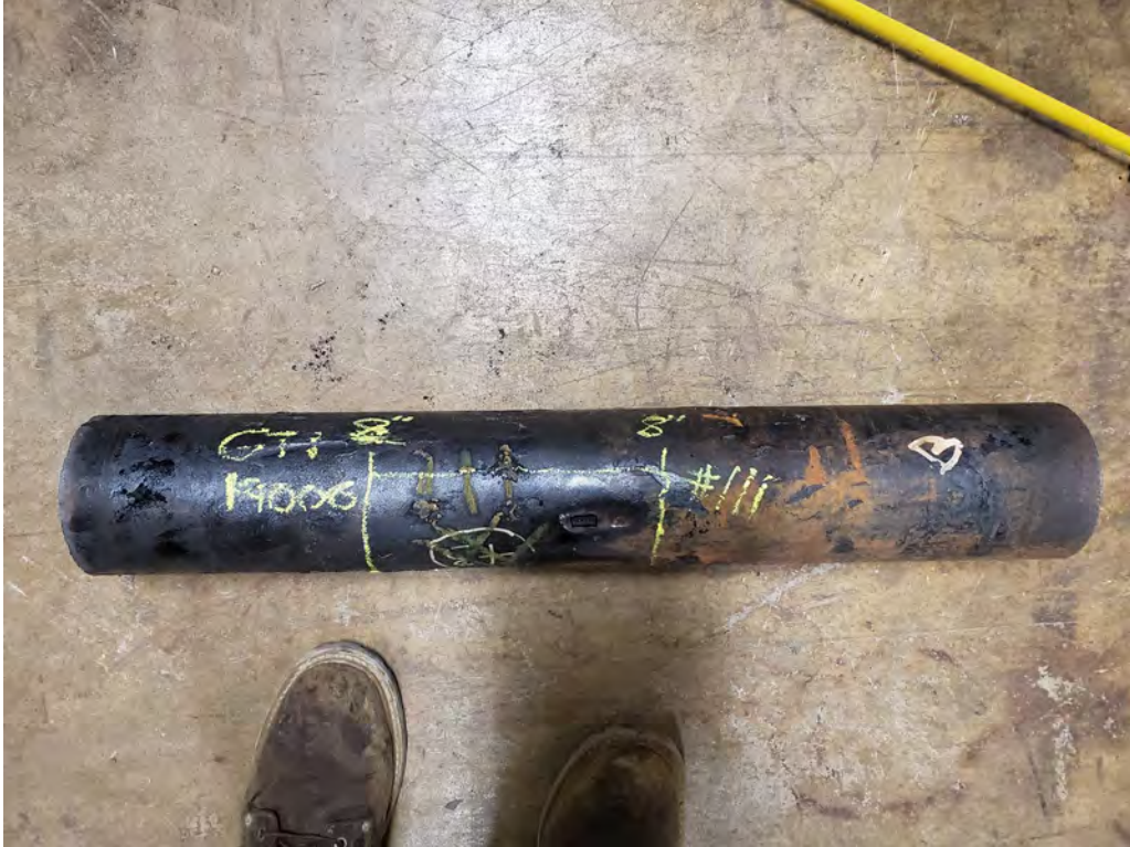
Figure 30: Test locations and overview of Sample 111.
