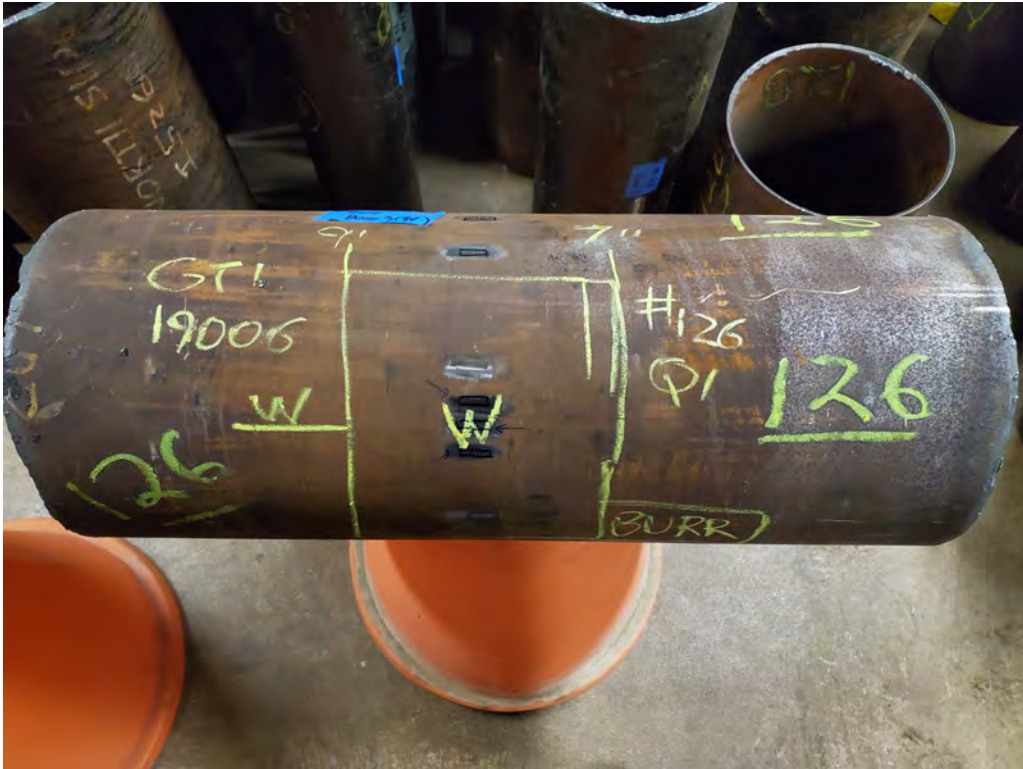
Figure 44: Test locations and overview of Sample 126.
