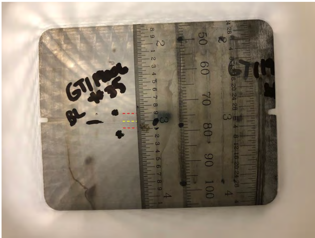
Figure 5: Examination of etched heat-affected-zone (HAZ) on the outer surface of the ERW seam for Sample 035. The boundaries of the etched HAZ are shown in dashed red lines and the bondline is shown by the dashed yellow line. The normalized HAZ width (measured width / wall thickness) is approximately 0.20 \text{ in} / 0.25 \text{ in} = 80\% .
