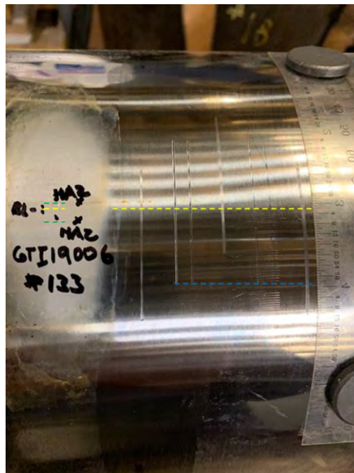
Figure 33: Examination of etched heat-affected-zone (HAZ) on the outer surface of the ERW seam for Sample 133. The bondline is located approximately 0.875 inches from the start of the HSD test.
