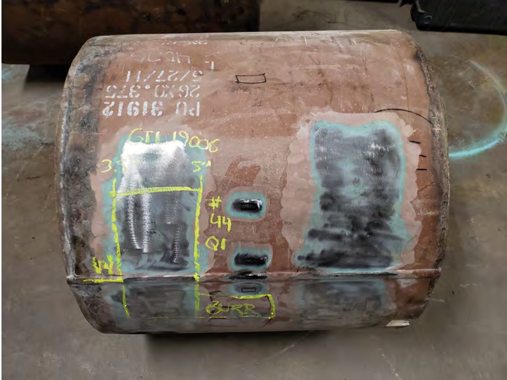
Figure 24: Test locations and overview of Sample 044.
