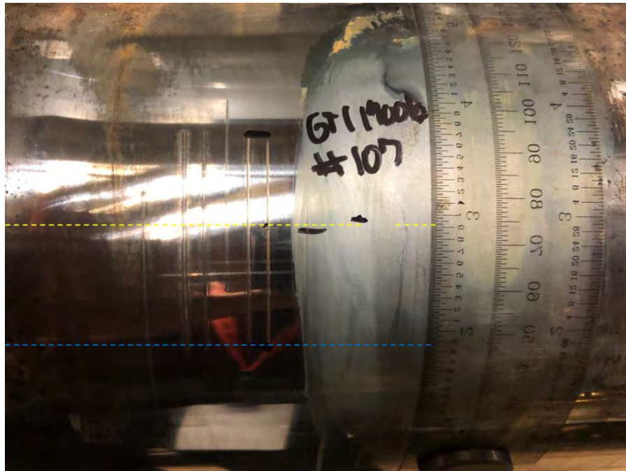
Figure 10: Examination of etched heat-affected-zone (HAZ) on the outer surface of the ERW seam for Sample 107. The bondline is located approximately 1.0 inch from the start of the HSD test.
