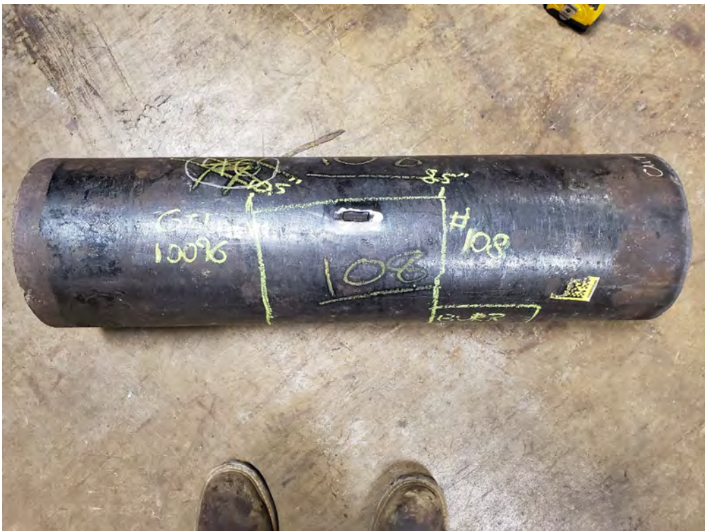
Figure 27: Test locations and overview of Sample 108.
