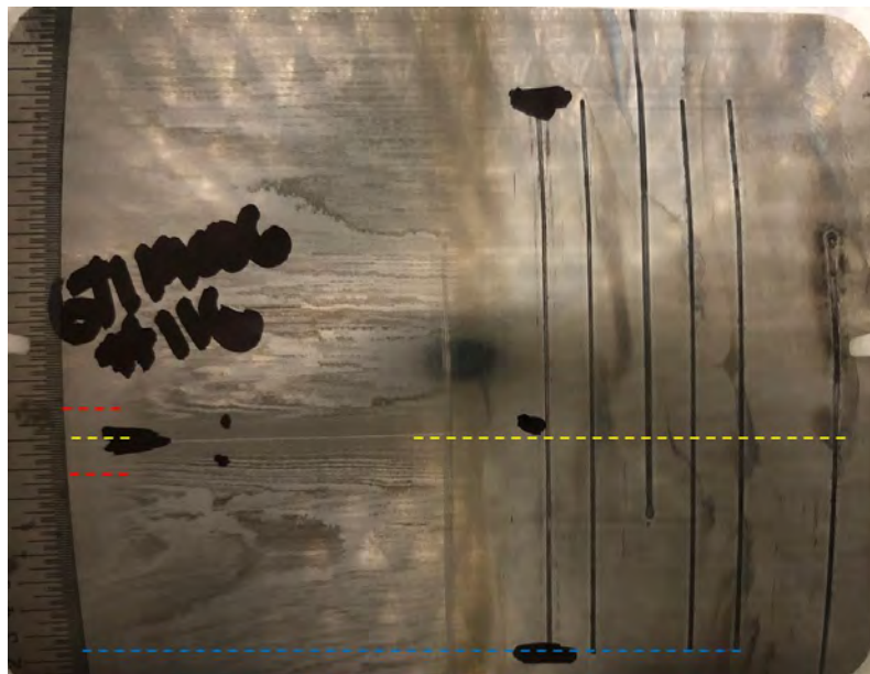
Figure 21: Examination of etched heat-affected-zone (HAZ) on the outer surface of the ERW seam for Sample 116. The bondline is located approximately 0.75 inches from the start of the HSD test.
