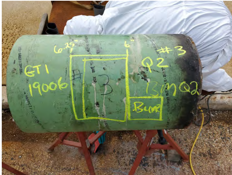
Figure 1: Test locations and overview of Sample 003.
