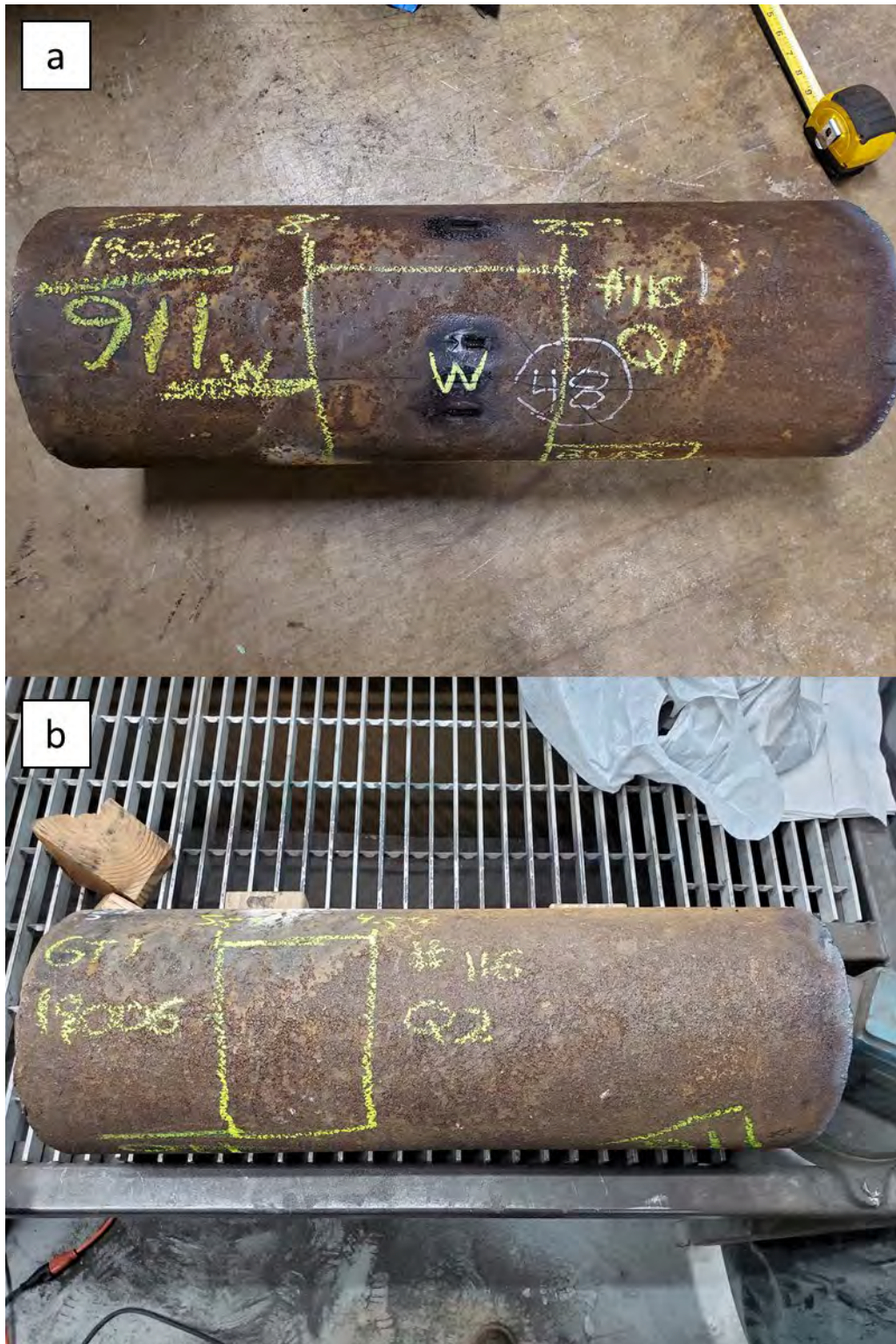
Figure 35: (a) Test location Q1 on ERW seam and overview of Sample 116; (b) Test location Q2 and overview of Sample 116.
