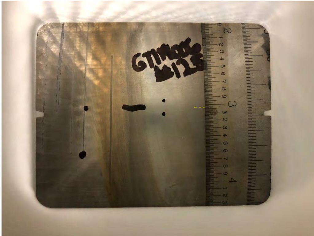
Figure 28: Examination of etched heat-affected-zone (HAZ) on the outer surface of the ERW seam for Sample 125. The bondline is shown by the dashed yellow line. There was no presence of a HAZ as a result of a complete normalization process indicative of HFN-ERW seams.
