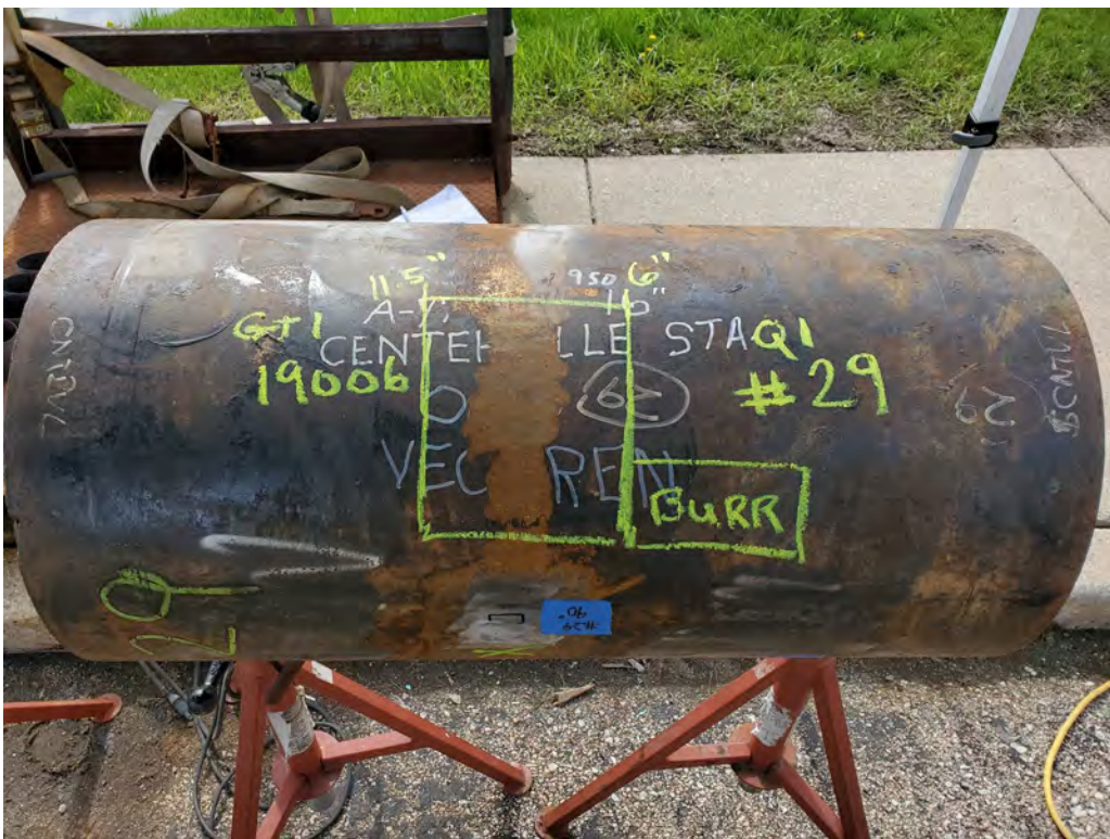
Figure 14: Test locations and overview of Sample 029.
