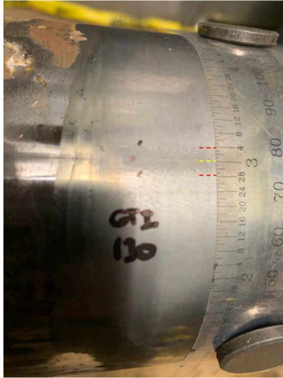
Figure 30: Examination of etched heat-affected-zone (HAZ) on the outer surface of the ERW seam for Sample 130. The boundaries of the etched HAZ, which blends into the contact lines, are shown in dashed red lines and the bondline is shown by the dashed yellow line. The normalized HAZ width (measured width / wall thickness) is approximately 0.25 \text{ in} / 0.20 \text{ in} = 125\% .
