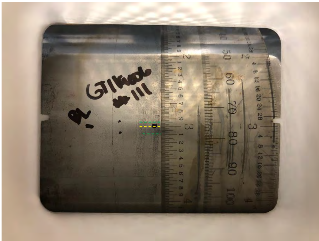
Figure 11: Examination of etched heat-affected-zone (HAZ) on the outer surface of the ERW seam for Sample 111. The edges of an inner hourglass HAZ surrounding the bondline are shown by the dashed green lines and the bondline is shown by the dashed yellow line. There is no presence of a larger, outer HAZ as a result of a normalization process indicative of HFN-ERW seams.
