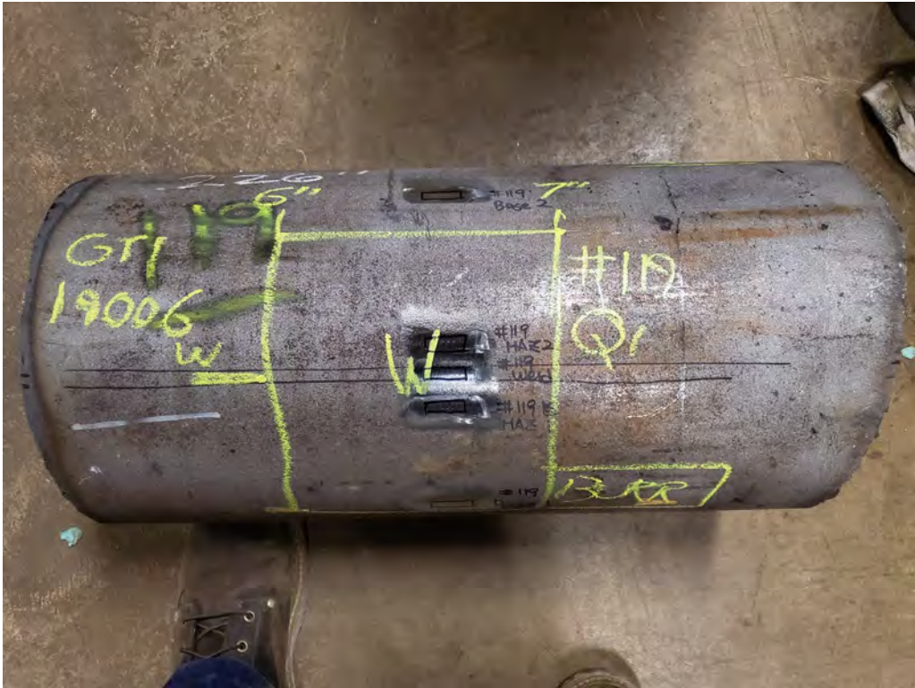
Figure 38: Test locations and overview of Sample 119.
