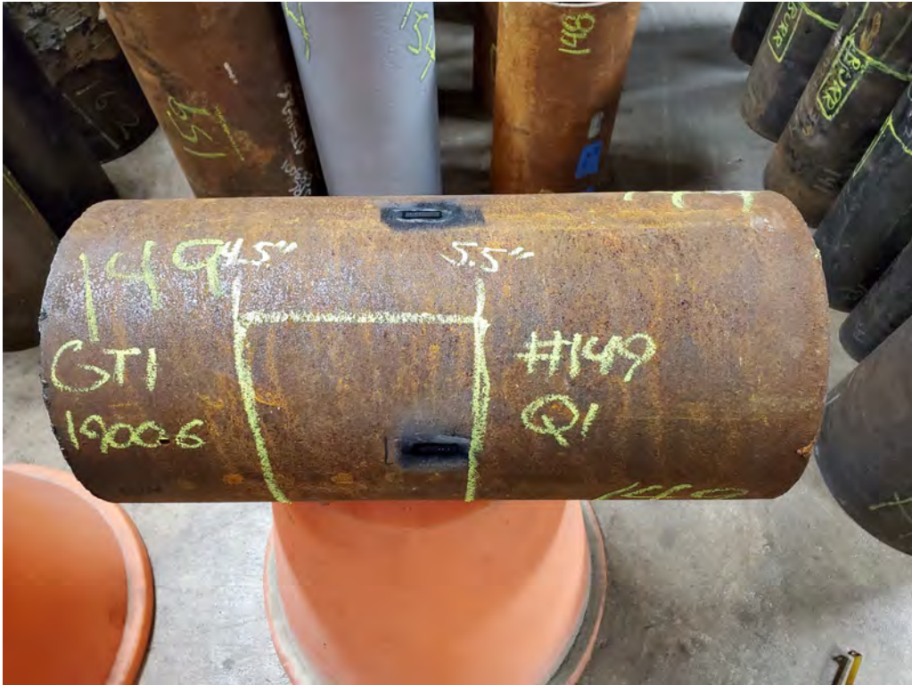
Figure 63: Test locations and overview of Sample 149.
