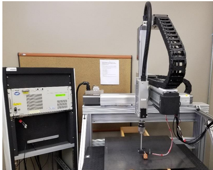
FIGURE 5. EPSON 3-STAGE SCANNING ROBOT WITH FLAT PLATE MREC.
