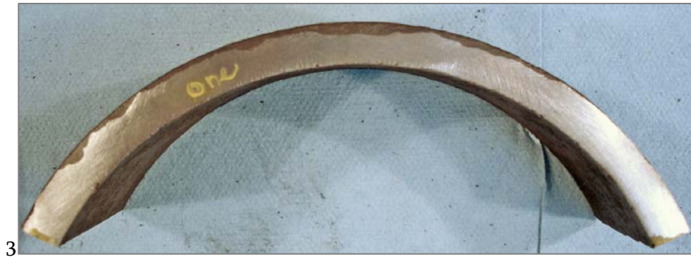
Figure 40. Dark, graphite corrosion on the exterior of a cast iron gas main.
