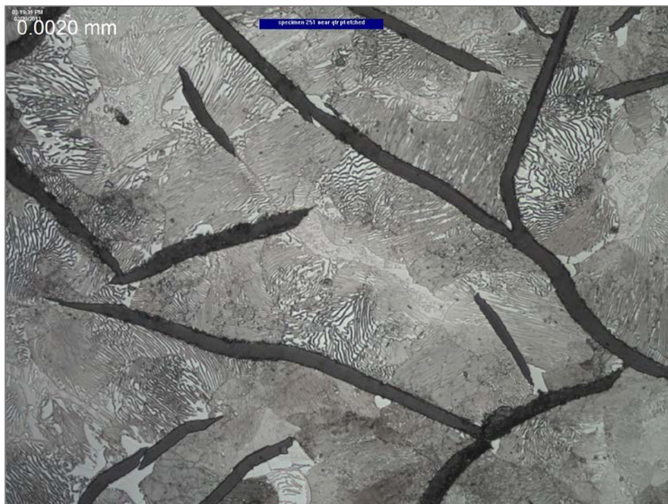
Figure 14. Etched gray cast iron microstructure, primarily pearlite.
