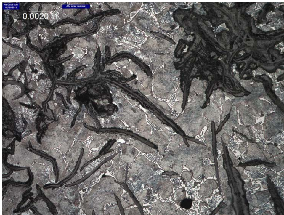
Figure 44. Example of microstructure of graphitic corrosion showing dealloyed regions around the large graphite flakes, i.e. expanded dark areas.
