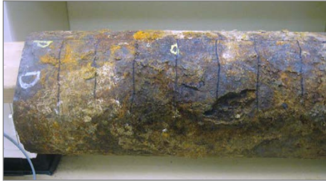
Figure 6. Cast iron gas pipe corrosion.
