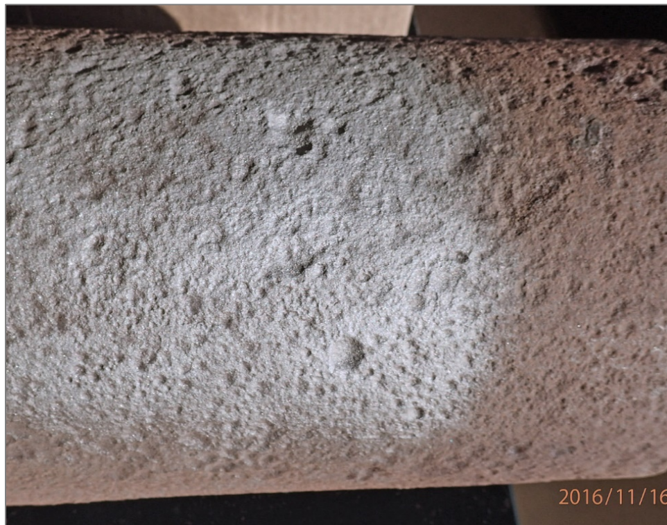
Figure 72. Severely corroded CI pipe after grit blasting
