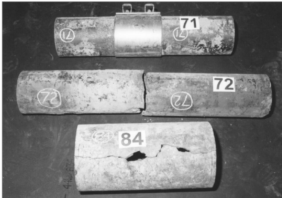
Figure 31. Longitudinally cracked (84), circumferentially cracked (72), and temporarily repaired, clamped (71) pipes.
