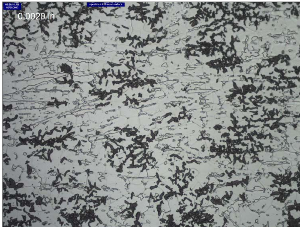
Figure 23. Etched gray cast iron microstructure. The white, horizontal banded structure is cementite and dispersed primarily at the ferrite boundaries.
