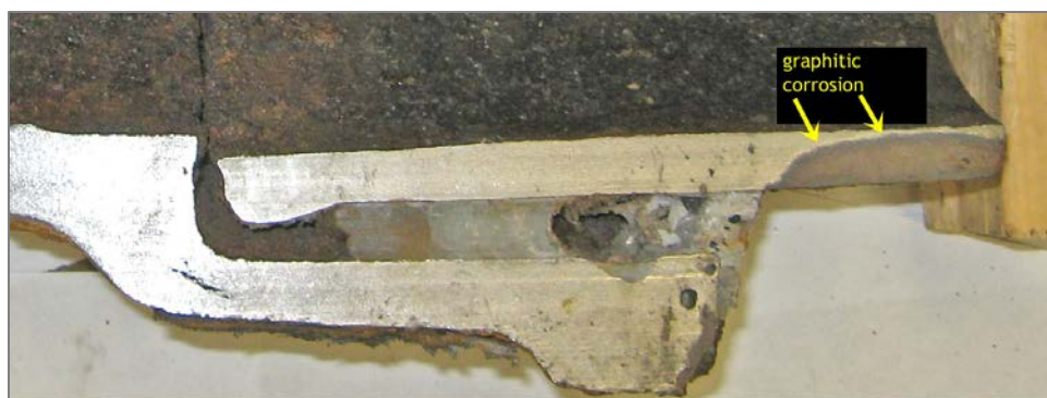
Figure 41. Dark, graphite corrosion near the entrance to a joint on the exterior of a cast iron gas main.
