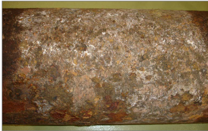
Figure 8. Cast iron gas pipe graphitic corrosion and pitting.
