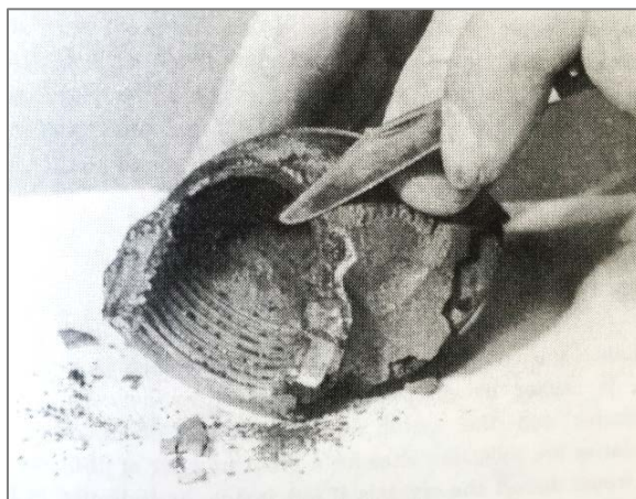
Figure 35. Graphitic corrosion of cast iron elbow.
