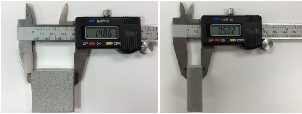
Figure 9. Dimensions of the sample to be tested.
