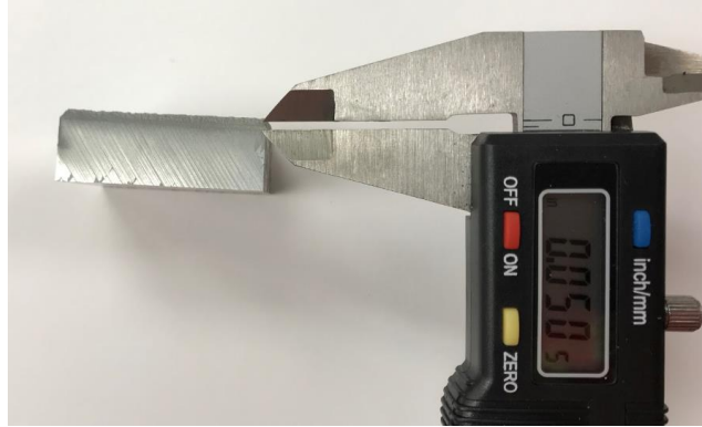
Figure 10. Measurement of coating thickness.
