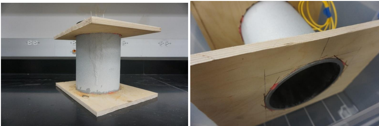
Figure 95. Coated pipe samples with wood board for isolating moisture soil from internal corrosion
