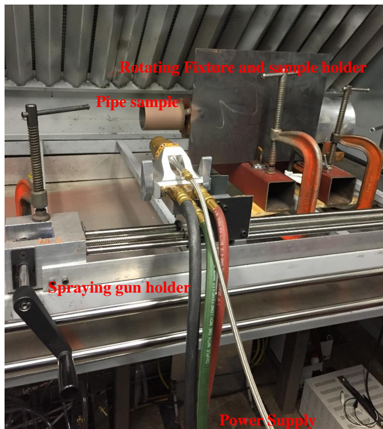
Figure 5. Automatic rotational fixture for pipe samples.
