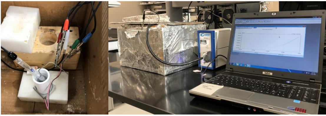
Figure 33. Accelerated electrochemical corrosion test setup.
