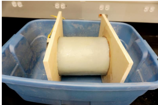
Figure 97. Pipe samples placed inside boxes for testing (left: wire arc sprayed Al-Zn coating, right: multiple-layer coating).
