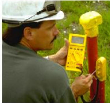
Figure 44. Field measurement example for pipe-to-soil potential 15 .
