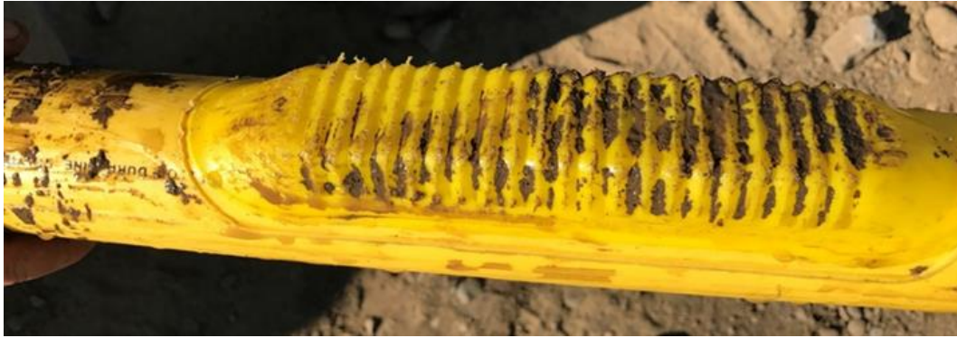
Figure 21: Condition of the PE pipe and housing after being pulled through the rocky ground
