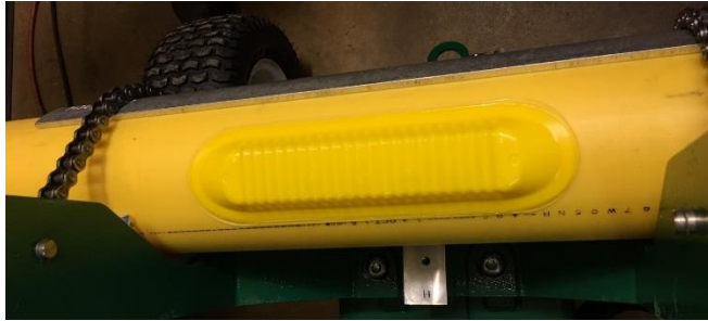
Figure 13: 4' Marker and housing fused to a 4" MDPE pipe
