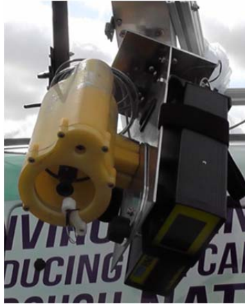
Figure 7. Conical-Scan Spinning RMLD. The transceiver is enclosed in a PVC housing. Both the transceiver and the RMLD electronics were rotated when performing a scan.
