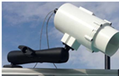
Figure 6. Side Scanning RMLD in fixed configuration. The commercial transceiver is further ruggedized using a PVC housing. Laser and electronic board are located inside the vehicle.
