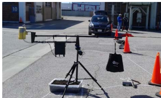
Figure 8. Stationary cylindrical-Scan Spinning RMLD performing cylindrical scans. This setup shows a calibrations setup with a plastic tub full of dirt and an embedded plastic tubing for calibrated gas releases.
