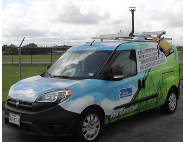
Figure 22. FLUX Mobile equipped with spinning and side-scanning RMLDs and anemometer.
