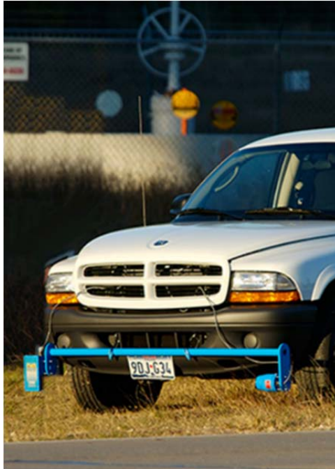
Figure 11. Optical Methane Detector (in blue).
