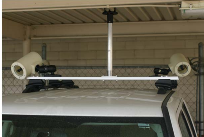
Figure 24. Advanced Mobile Unit showing two installed side scanning RMLDs and Anemometer.
