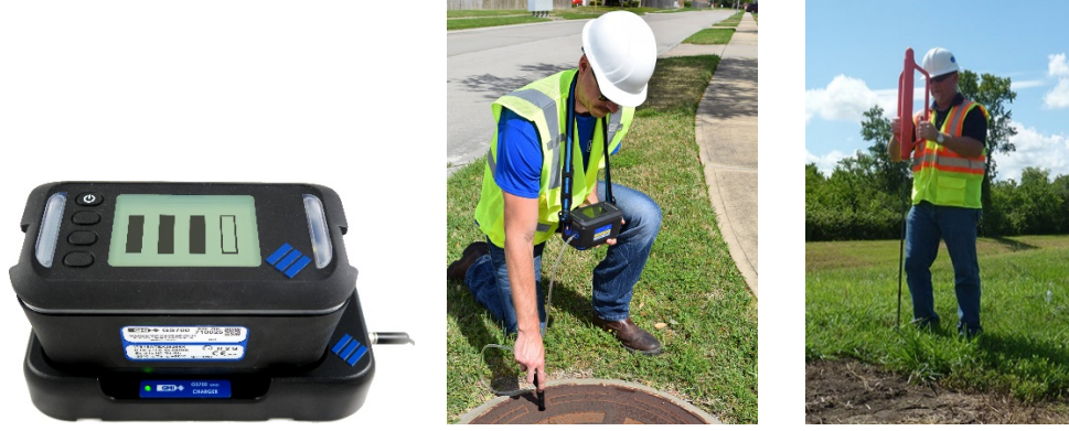
Figure 13. Gasurveyor 700 Multi-Gas Detector and plunger bar to perforate ground (right).
