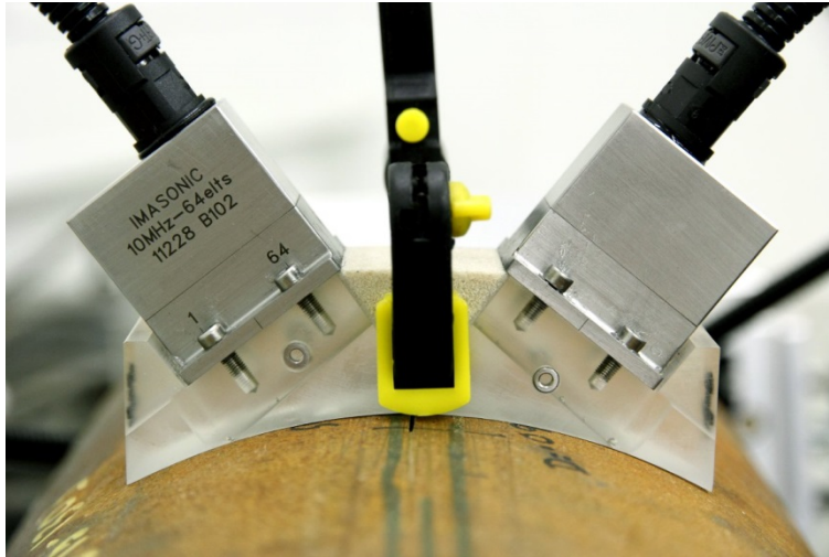
Figure 1-1. Laboratory test setup for IWEX on seam welds
