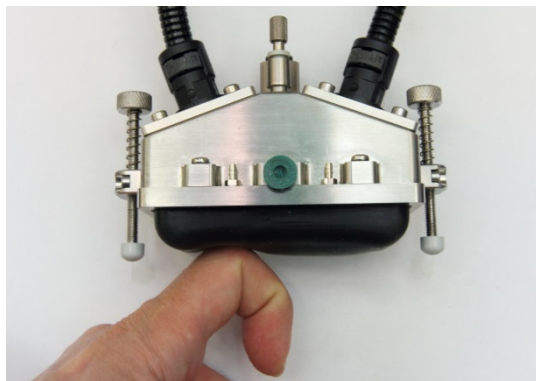
Figure 6-45: Flexibility of the water-filled wedge when pushed.
