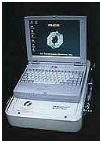
Figure 4. Photograph showing PR4500 data acquisition system and monitor.
