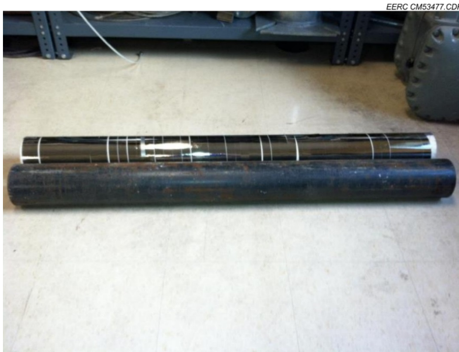
Figure 5. Photograph of PVC pipe wrapped in amorphous foil (top) and standard iron pipe (bottom).
