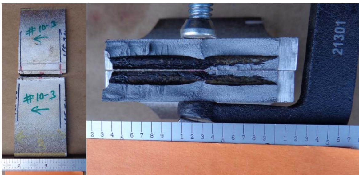
Figure 46. SWA #8-2, break location and fracture surface
