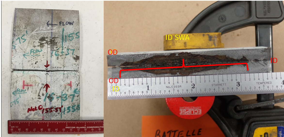
Figure 4. SWA #1, Break location and fracture surface
