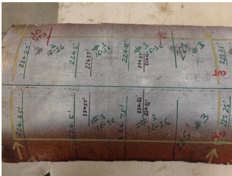
Figure 13. Break location marked on SWA #3
