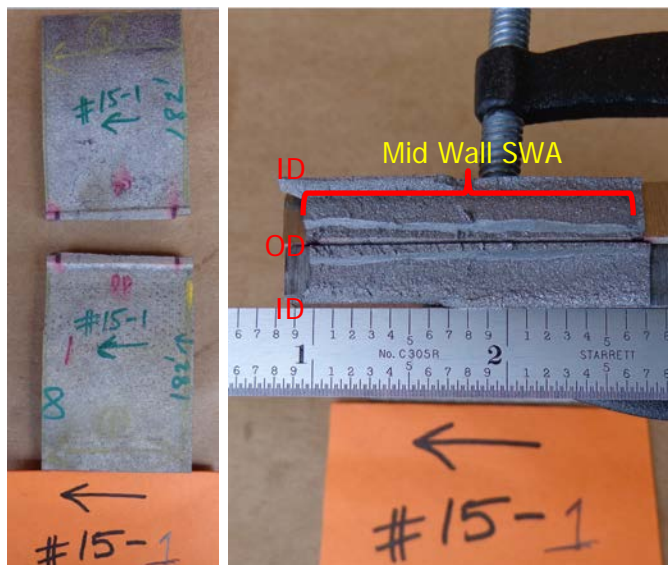
Figure 74. SWA #15-1, break location and fracture surface
