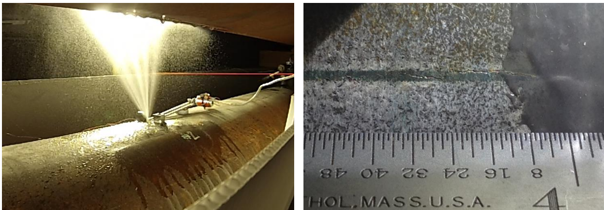
Figure 23: Feature #2 Leaking While Pipe at Approximately 1500 psi (left) and Then Shown after De-pressurized (right)
