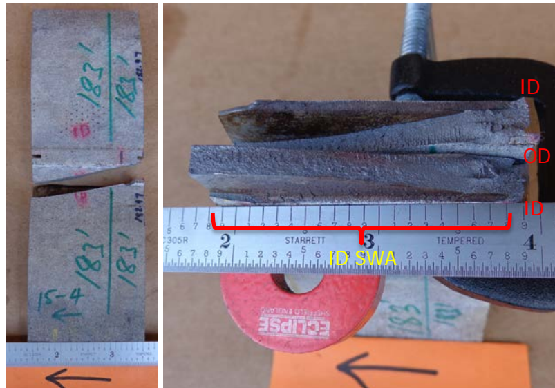
Figure 76. SWA #15-3, break location and fracture surface
