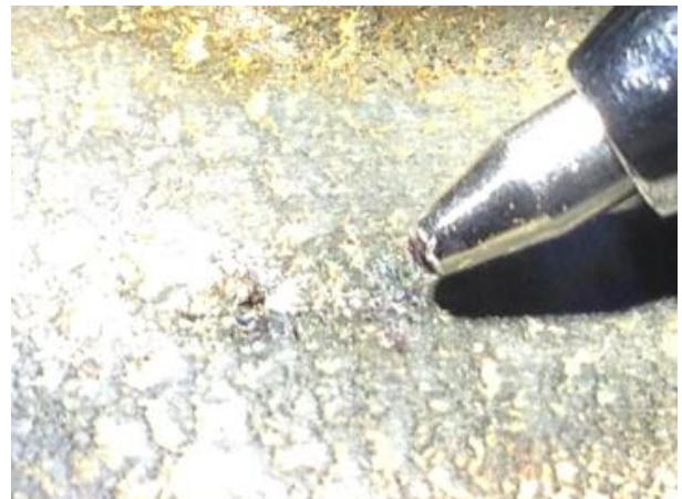
Figure 20: Feature #1 Leaking While Pipe at Approximately 1420 psi (left) and Then Shown after De-pressurized (right)
