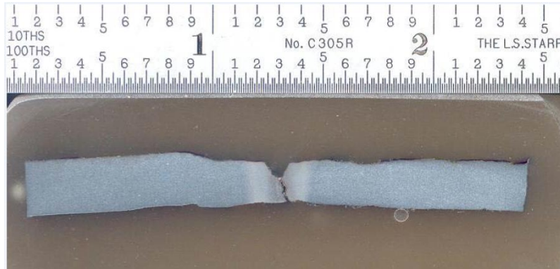
Figure 13: SSWC Example with U-Shaped Selective Corrosion [1]
