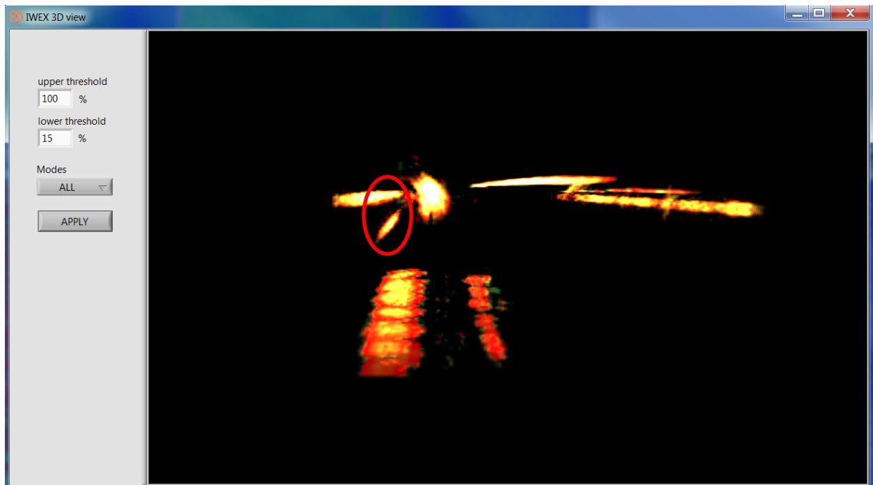
Figure 48. Part 116050, 3025 + 77mm, D 0.0 – 1.1, H 1.1mm, US 270 Side with flow OD surface LOF
