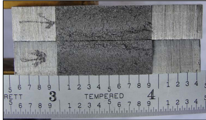
Figure 114. Fracture surface of Defect #3. The defect appears to be 0.1-in (2.5 mm) deep from the ID surface
