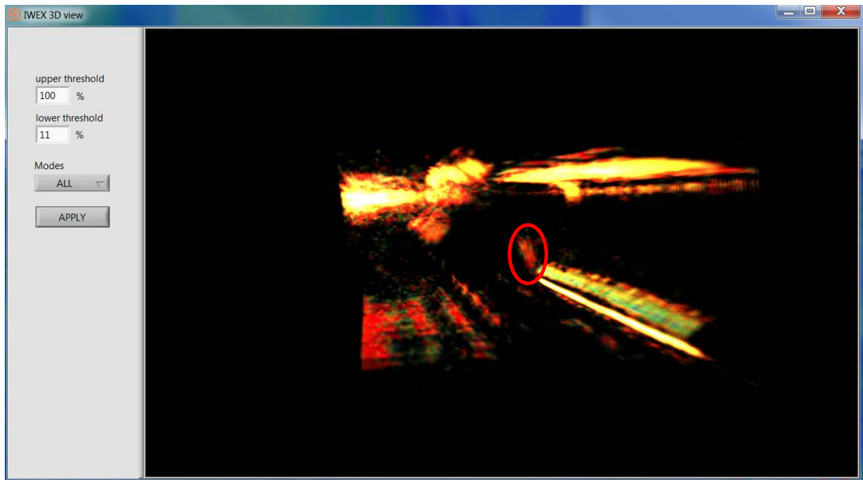
Figure 59. Pipe Sample 159070, 1258 + 5mm, D 1.6 – 2.9mm, H 0.5mm, DS 90 side with flow LOF
