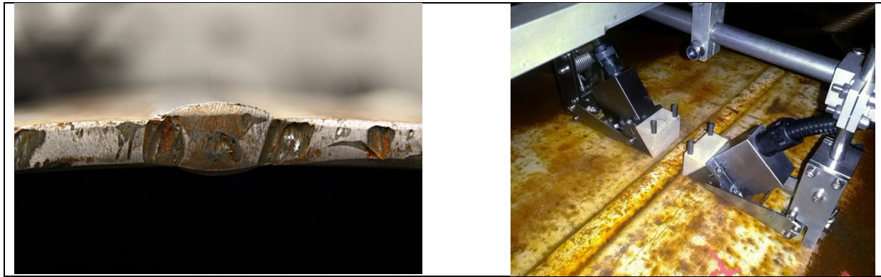
Figure 96. Cross-sectional view of the weld (left); measurement setup (right)
