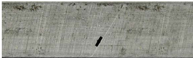
Figure 12. Test block with a 2 mm notch with an angle of 30° with respect to the vertical axis.
