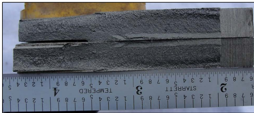
Figure 112. Fracture surface of Defect #2, the fracture broke in the intended plane for about half the fracture surface.
