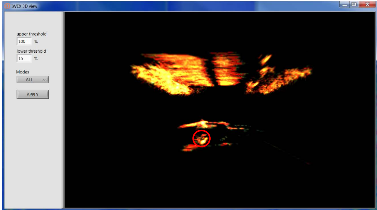
Figure 69. Pipe Sample 159070, 744 + 5.5mm, D 6.1 – 7.4, H 1.3mm, US 270° with flow ID surface LOF
