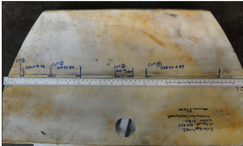
Figure 110. The 26-in diameter coupon with markings showing locations of the flaws
