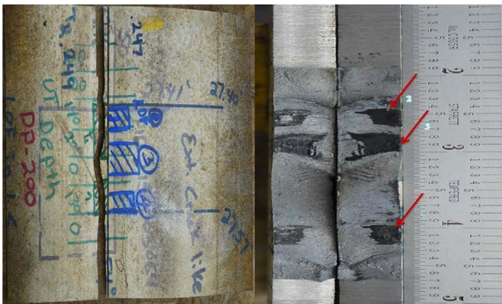
Figure 91. Lack of Fusion defects on Fracture Surface
