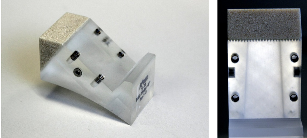
Figure 5. Wedges used for the seam weld inspection using IWEX: side view of a wedge designed for 8-in pipe showing the curvature of the wedge bottom (left), top view showing the shape of the conical lens included in the wedge (right).
