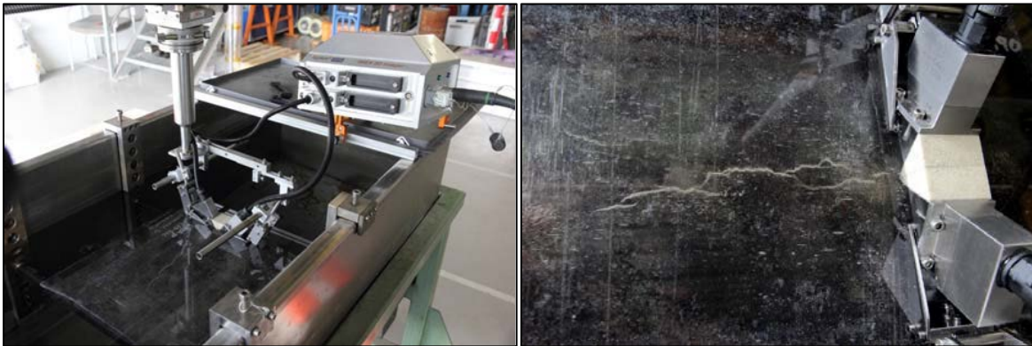
Figure 36. Measurement setup with the pipe coupon being submerged in water (left); position of the two array probes on wedges with respect to the area of interest (right).
