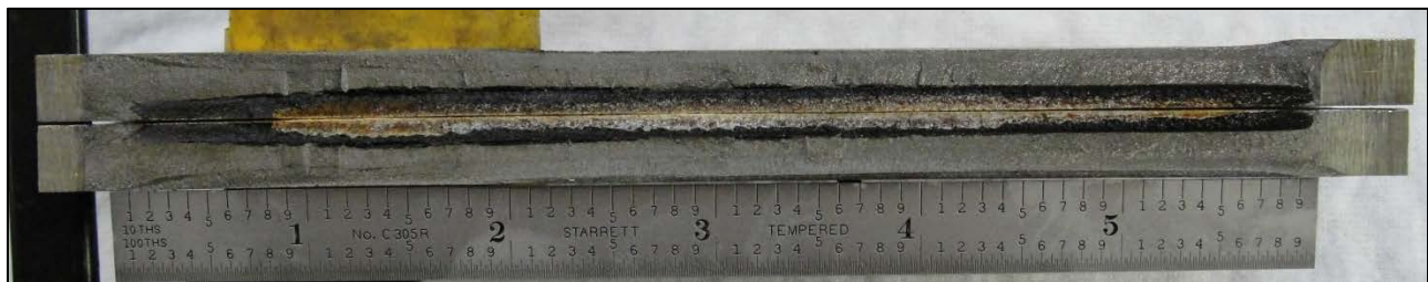
Figure 115. Fracture surface of Defect #4, the largest defect with the internal surface breaking defect. The defect appears to be about 0.15-in (3.8 mm) deep from the ID surface.
