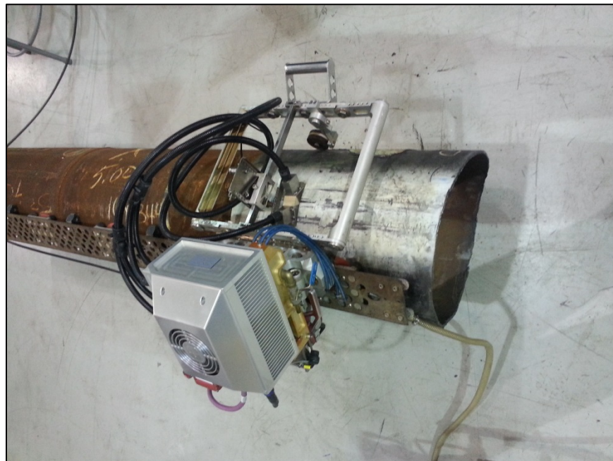
Figure 77. Initial scanning system: modified LNG tank scanner
