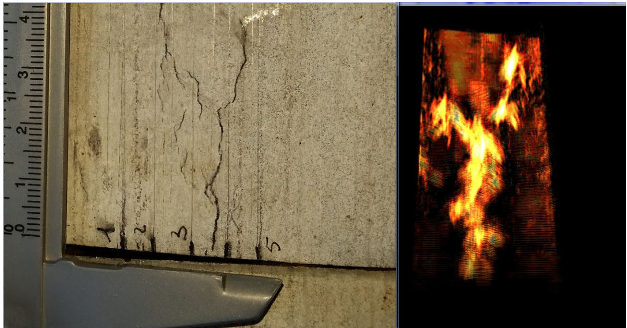
Figure 106. Mosaic image of C-scan representation over pipe sample photos
