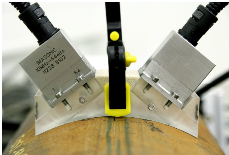
Figure 1. Laboratory test setup for IWEX on seam welds
