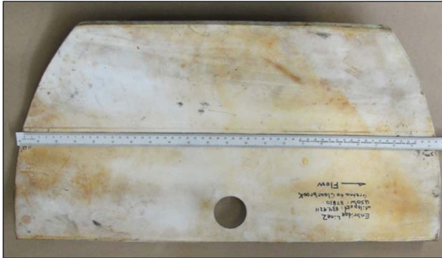
Figure 109. A 26-in diameter coupon with visible flaw on the ID seam weld
