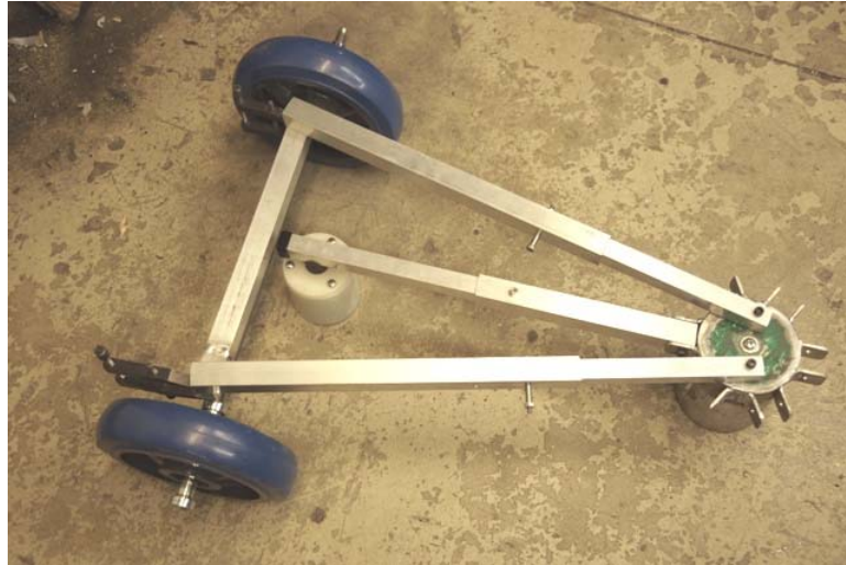
Figure 11 Partially fabricated system carriage with wheels and array assembly.
