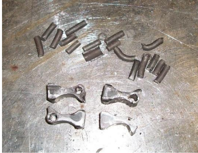
Figure 61 View of the pieces of the hammers and rods recovered from the source after initial testing.
