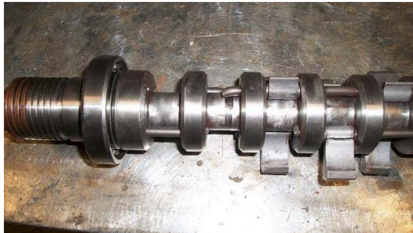
Figure 60 Photograph of the damaged hammer assembly recovered after initial source testing. Both failed rods and hammers can be seen. Failures were most likely due to counter-rotation of the hammers against the anvils, as explained in the text.
