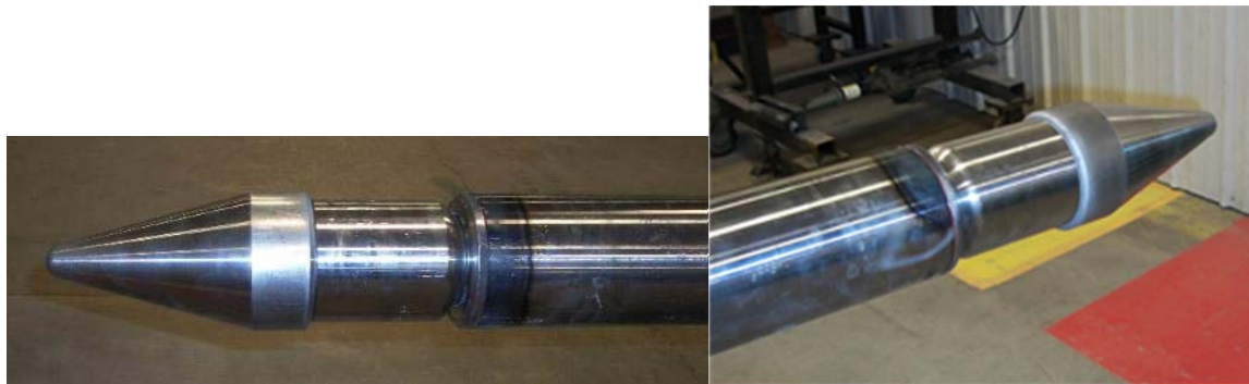
Figure 51 Photograph of the source showing the uphole rod-in-rod design. The inner rod turns the hammer assembly.
