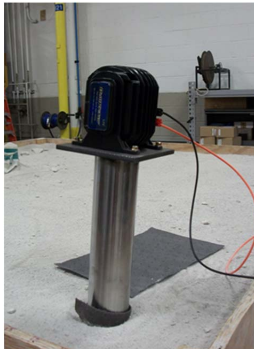
Figure 15 Photograph of the surface seismic actuator transducer. Fixtures have been made that allow axial or transverse motion to be applied to the ground.
