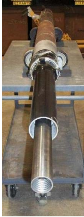
Figure 51 Photograph of the source showing the uphole rod-in-rod design. The inner rod turns the hammer assembly.
