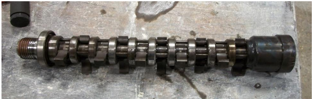
Figure 63 View of the hammer assembly recovered after the completion of trials. Other than damage to one hammer, no wear or damage could be found on the source.
