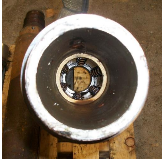
Figure 62 View down the interior of the outer head casing showing anvils. This photo was taken after operating procedures were corrected and trials conducted. There is essentially no wear on the anvils resulting from testing.
