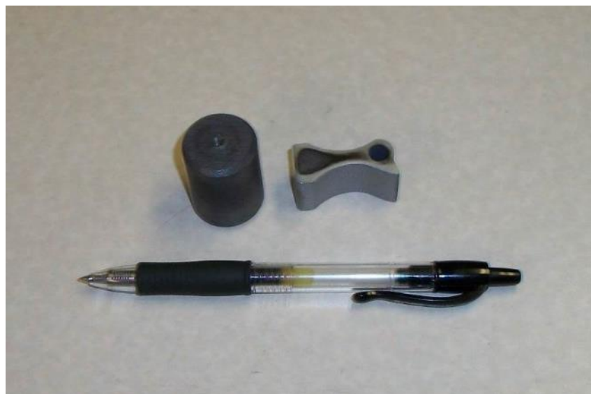
Figure 48 Close-up of the anvil (left) and hammer (right) to be used in the enhanced acoustic source. A ball point pen is included for scale.
