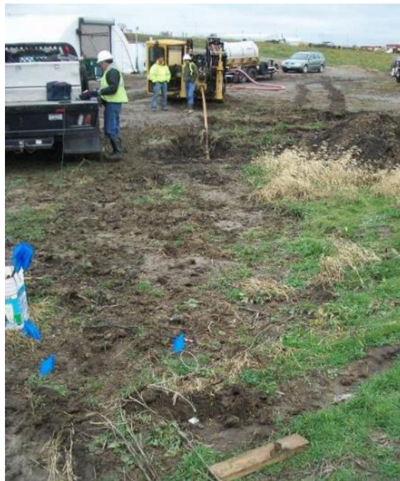
Figure 54 Data collection setup. Accelerometers mounted on aluminum cubes were placed at varying distances from the source as its hammer assembly was rotated at 120 and 240 rpm.
