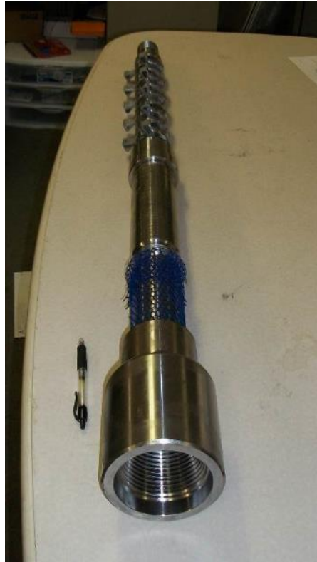
Figure 49 Photograph of the coupling/drive assembly for the acoustic source. The inner drive rod of the dual rod system will be used to rotate the near fitting, resulting in the hammer rotation and impacts.
