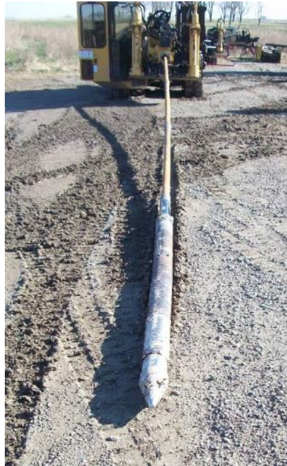
Figure 53 Photograph of the source during initial testing. During this test the hammers were rotated up to a maximum of 270 rpm with no failures or jams.
