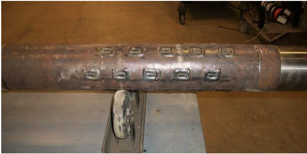
Figure 50 Photograph of the hammer section of the acoustic source after the hardened anvils have been welded in place. Diameter of this section is 5.5 inches.
