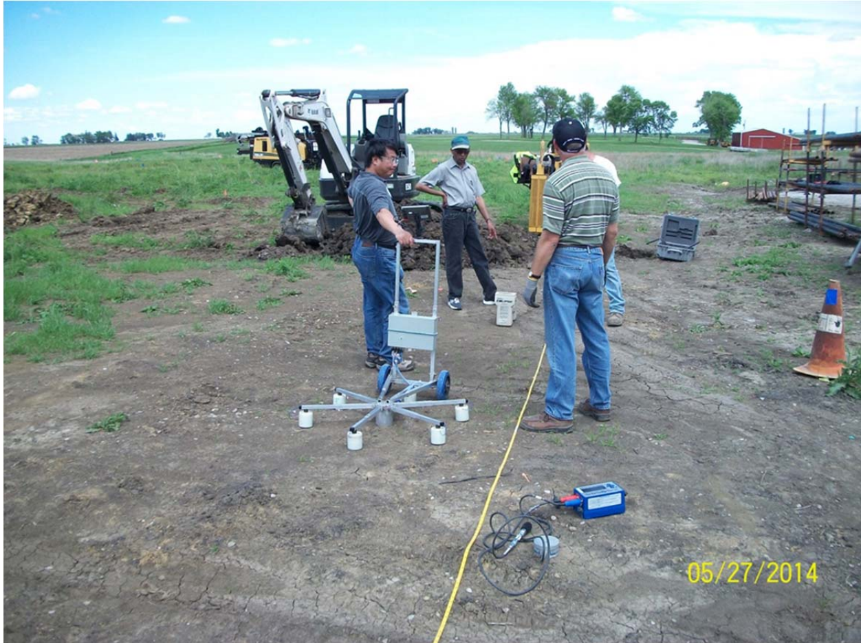
Figure 18 Acoustic system testing in the local area.
