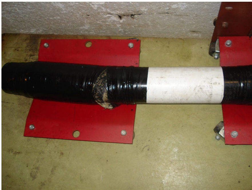
Figure 25 - Flexpipe sample in long-term cyclic test No. 4-A
