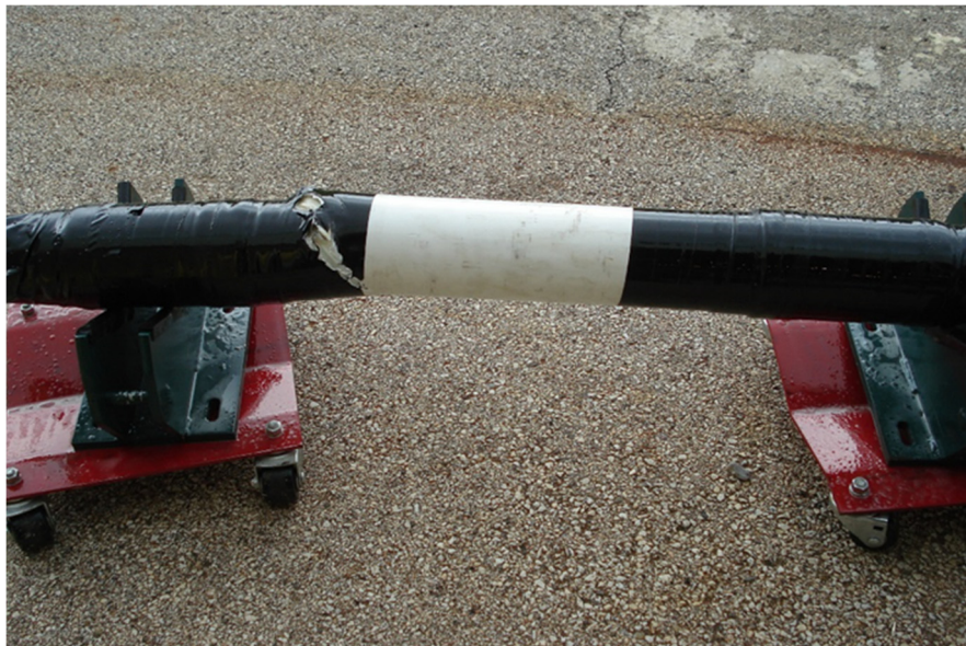
Figure 23 - Flexpipe sample in short-term rupture test No. 1
