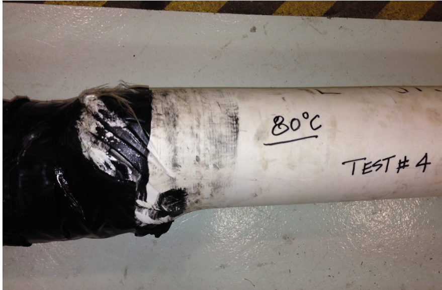
Figure 31 - Flexpipe sample after elevated temperature cyclic test No. 4
