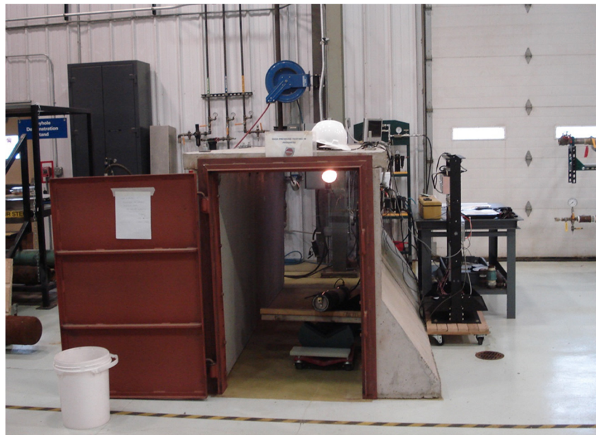
Figure 15 - The concrete chamber for room-temperature tests
