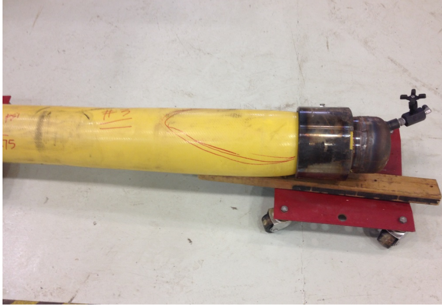
Figure 20 - Primus liner, sample leak at the bulge near the end connector, test No. 3
