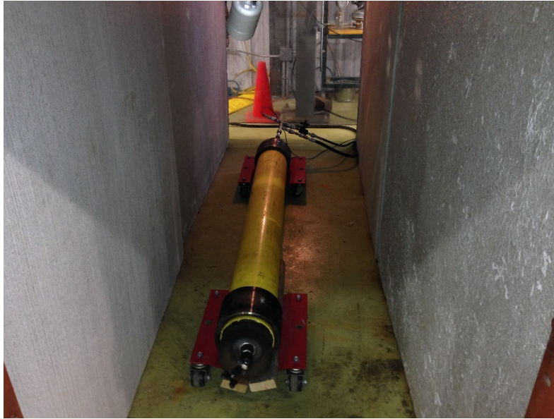
Figure 13 - The Primus Line test sample with the end-caps in the test chamber
