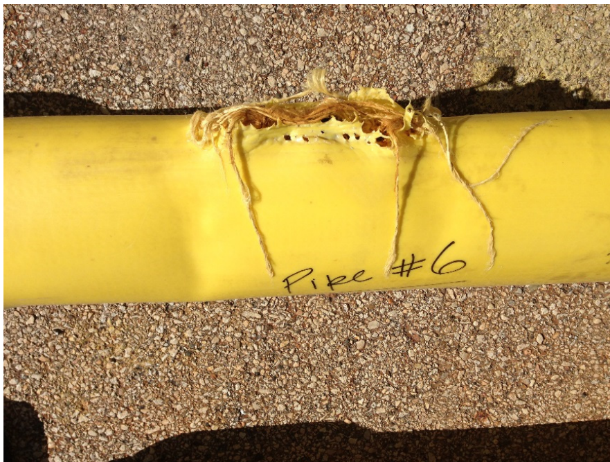
Figure 21 - Primus Liner, sample rupture at long-term cyclic test No. 6
