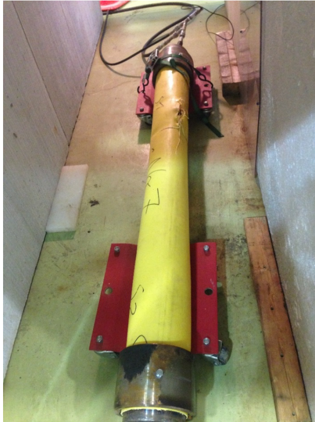
Figure 22 - Primus Liner, sample rupture at long-term cyclic test No. 7
