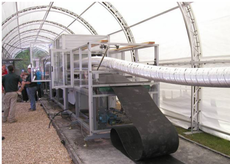
Figure 4 - Portable setup for the pipe fabrication
