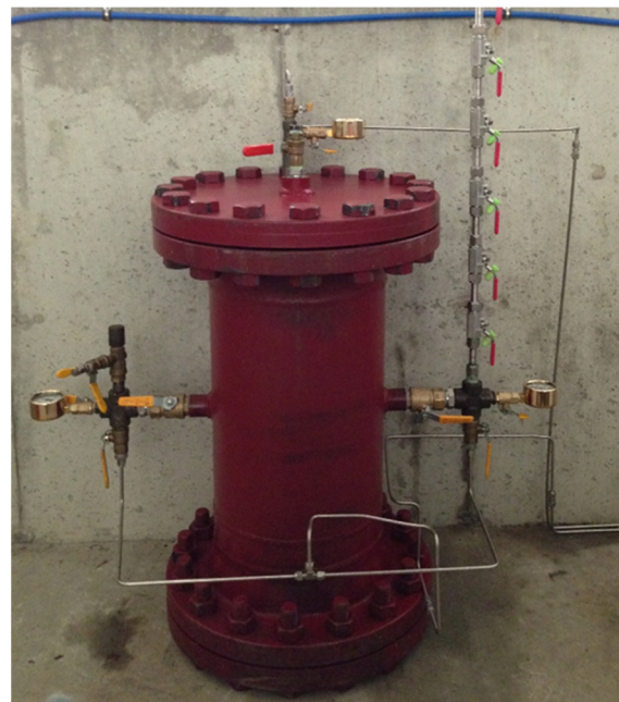
Figure 45 - The pipe specimen in the permeability test setup
