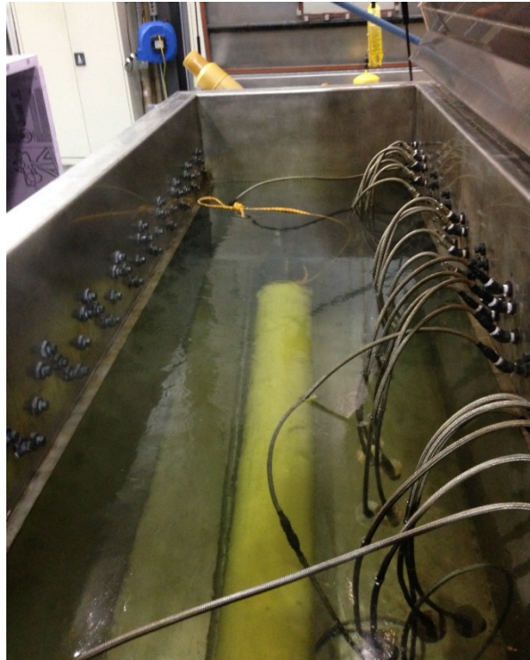
Figure 27 - The Primus Liner in the elevated-temperature test
