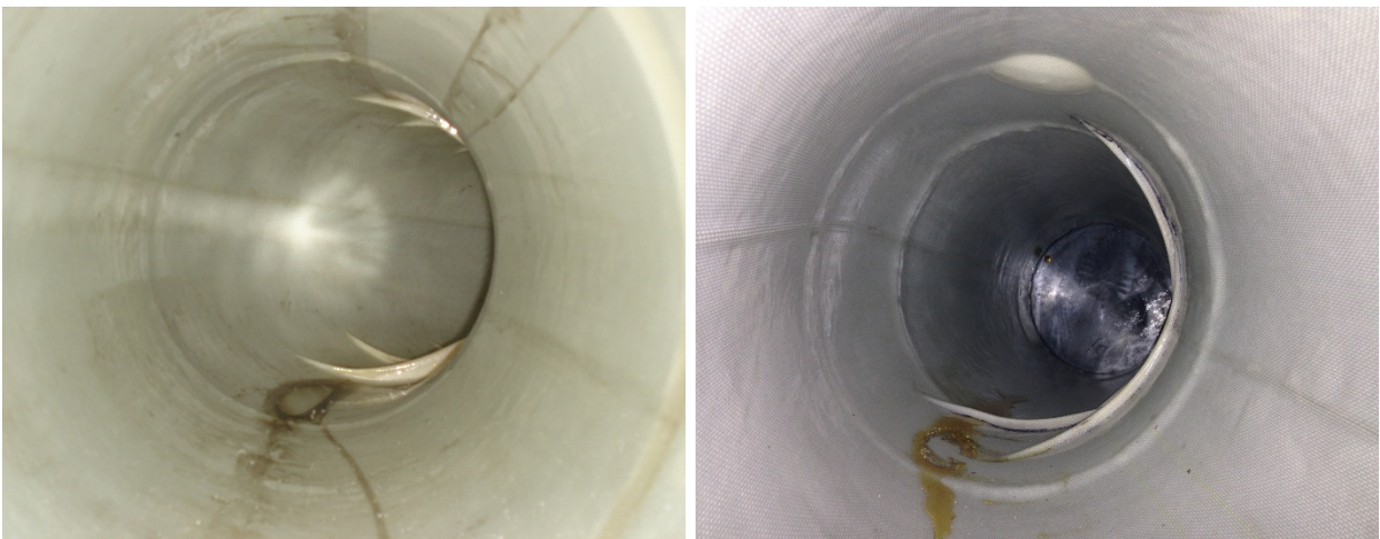
Figure 54 - Small delamination at the top after 350 psi depressurization
