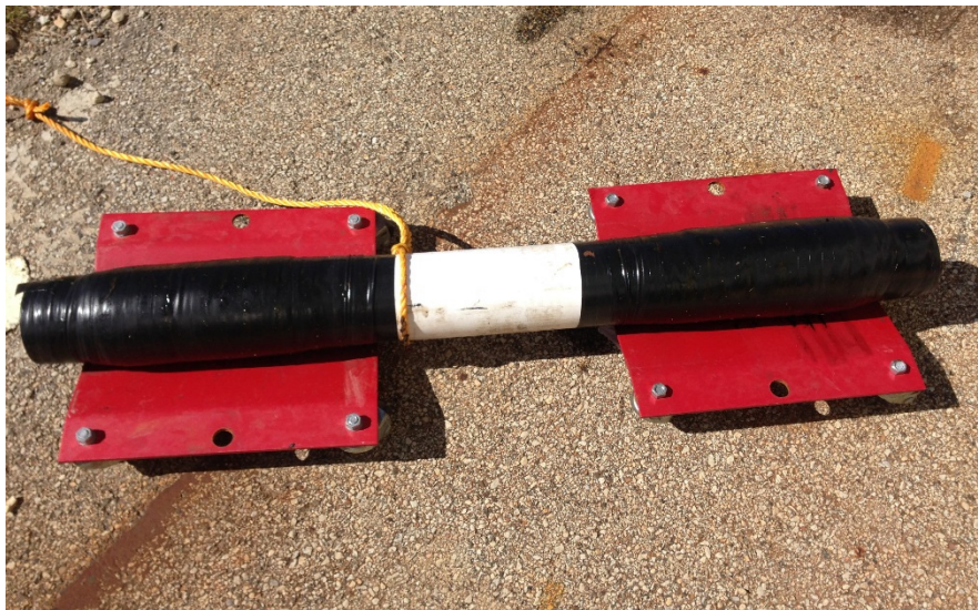
Figure 32 - Flexpipe sample after elevated temperature cyclic test No. 1-A
