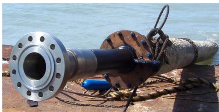
Figure 6 - Flanged end connection of the FlexSteel Pipe
