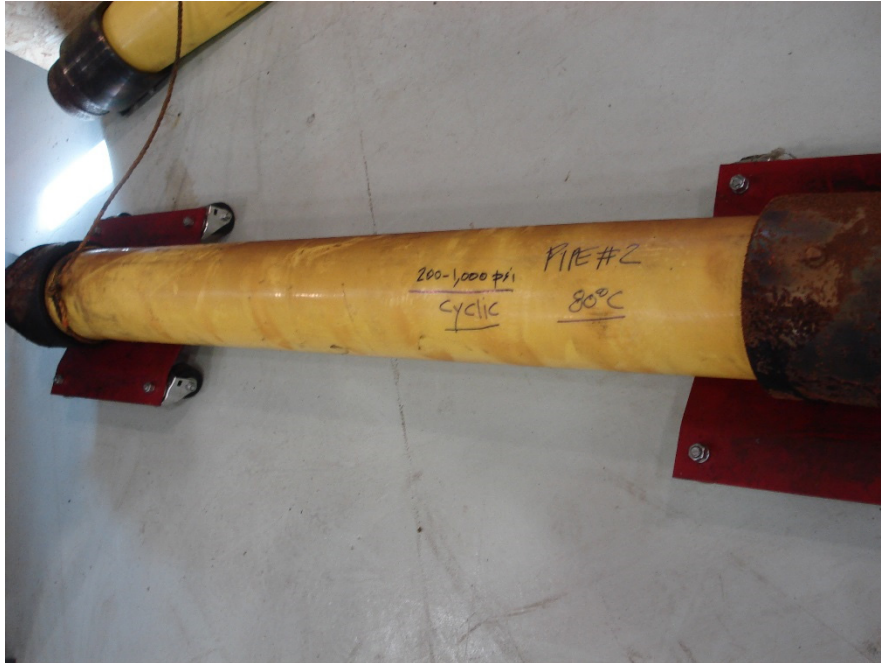
Figure 29 - Primus sample at elevated temp cyclic test No. 2
