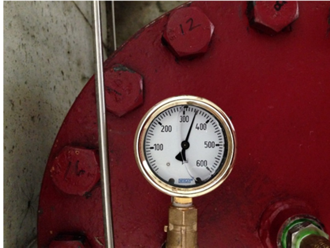
Figure 46 - Pressure gage for monitoring internal pipe pressure in the specimen
