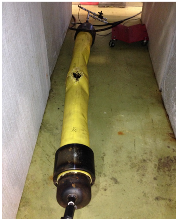
Figure 19 - Primus Liner, short-term rupture test, test No. 1
