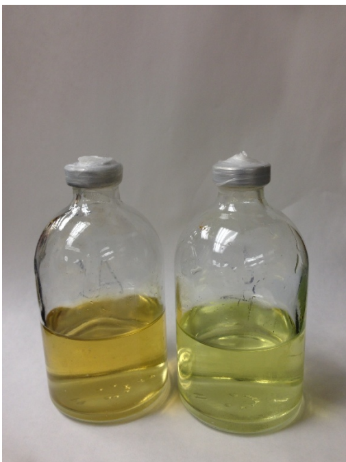
Figure 9-6. Left vial: 50 ml NRB medium and inoculated with 2 ml field sample solution incubated at 37°C for 15 days; Right vial: uninoculated original culture medium before incubation.
