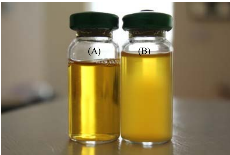
Figure 9-5. Color change of Phenol Red Dextrose medium due to: (A) pH and (B) bioactivity. The cloudiness is noticeable in the right vial.
