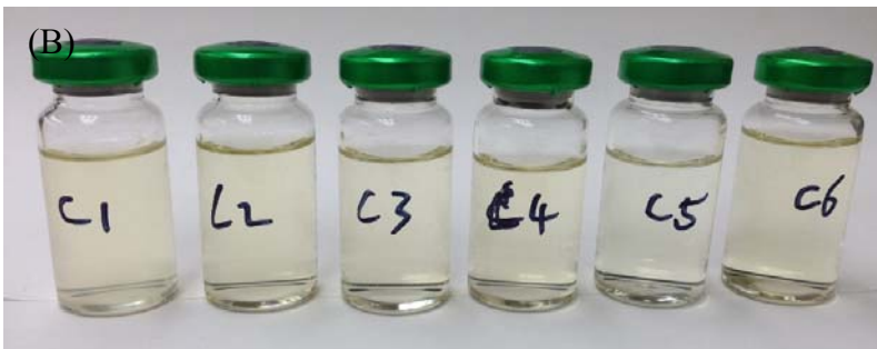
Figure 9-3. Vials of Standard Bacterial Nutrient Broth medium used to count GHB sessile cells in two biofilm consortia: (A) Consortium I and (B) Consortium II. The numbers 1 to 6 indicate the actual dilution.
