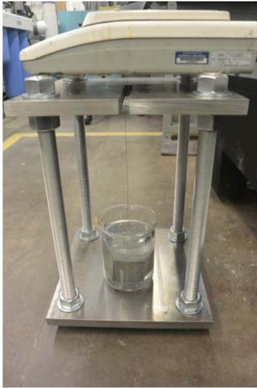
Figure. Setup to determine submerged mass.
