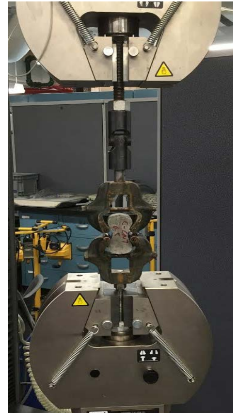
Figure. Tensile strength setup.
