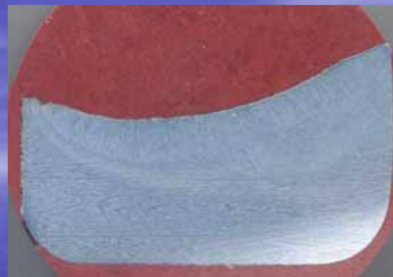
Longitudinal section macrograph showing the pool of a wet weld deposited with E6010 electrode
