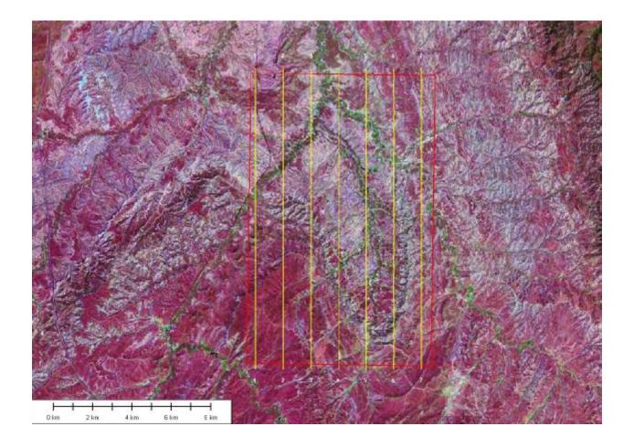
The seven flight lines that were required to image the entire NPR3\_RMOTC site are shown mosaiced together in the Figure 4 below. The images are shown in grayscale using one of the bands in the visible wavelengths.
