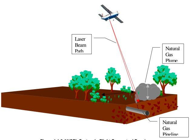
Figure 1.1.2 ANGEL System In-Flight Conceptual Drawing
