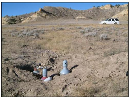
Site 2D/Site 1F – Three bottles (two with methane only, one with methane/ethane mix).
