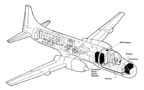
Figure 1.2.2 ANGEL Test Aircraft with Payload Installed
