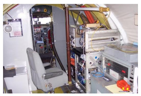
Figure 1.2.4 Airborne System Operator's Station in Test Aircraft
