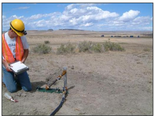
Site P2 – View of leak site and vegetation. The gas leak emits underground near the middle of the greasewood bushes.
