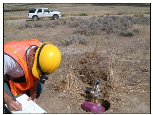
Site 2B – Underground leak located in the gravel area approximately 8 feet from bottle location.
