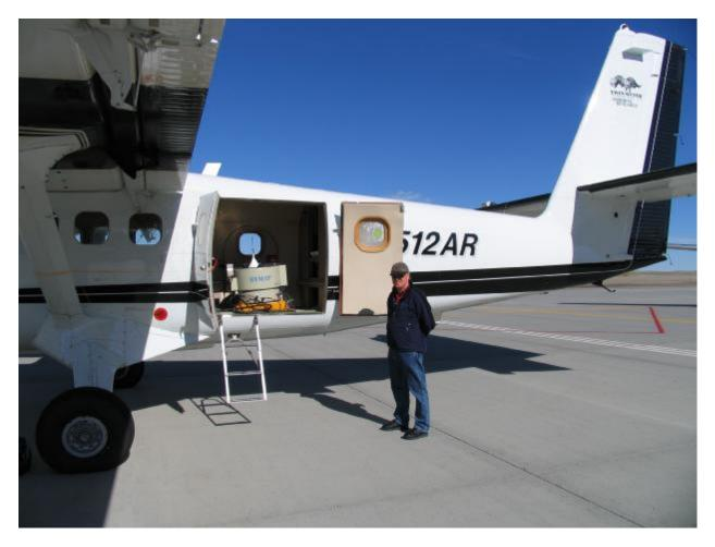
Figure 1 The HyMap sensor is white sitting on the stabilizing platform that is yellow inside the Twin Otter manned aircraft. Mike Hornibrook who is the HyVista operator is shown standing outside side the hatch doors.
