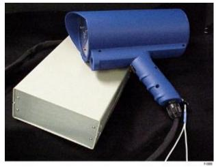
Figure 1. Remote methane leak detector alpha prototype unit.
