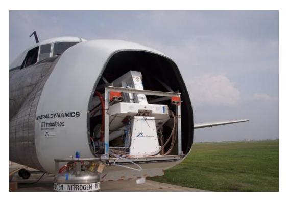
Figure 1.2.3 ANGEL Transceiver in Test Aircraft
