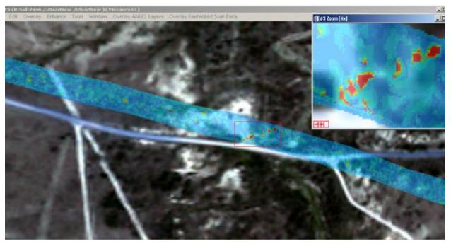
Figure 1.1.3 Visual Display of Natural Gas Emissions Detected By the ANGEL System on the Afternoon of September 17<sup>th</sup>, 2004 (Calibration Leak)
