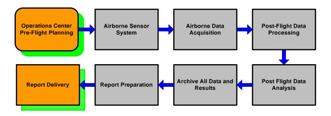
Figure 1.1.1 ANGEL System Block Diagram
